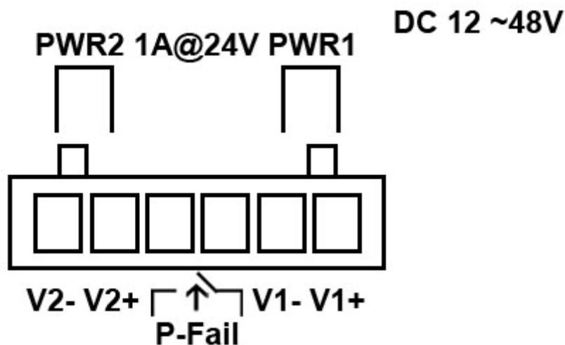
Figure 2.8: Pin Assignment of the Power Connector
