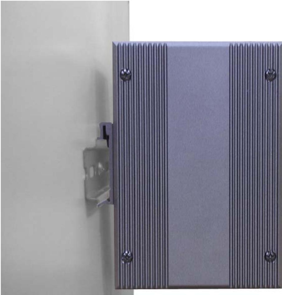
*Figure 2.7: Installation to DIN-rail Step 2*
