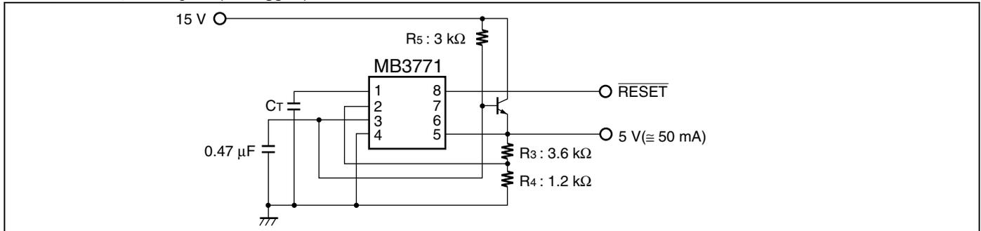
**8.10.3 5 V Reference Voltage Generation and 5 V Monitoring (No. 2)**
