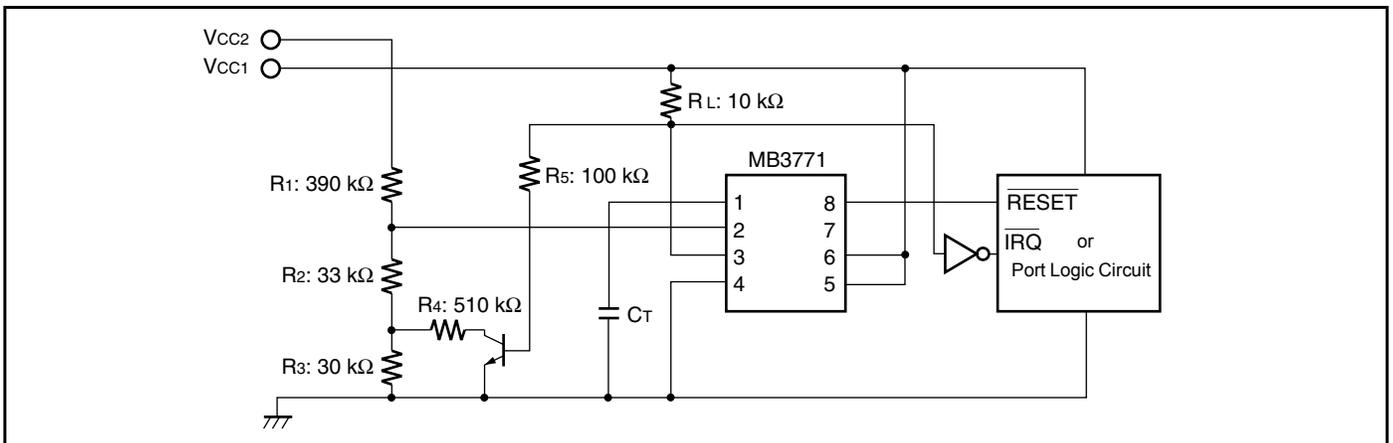
**8.6 5 V Power Supply Monitor with forced  $\overline{\text{RESET}}$  input ( $V_{CC} = 5 \text{ V}$ )**
