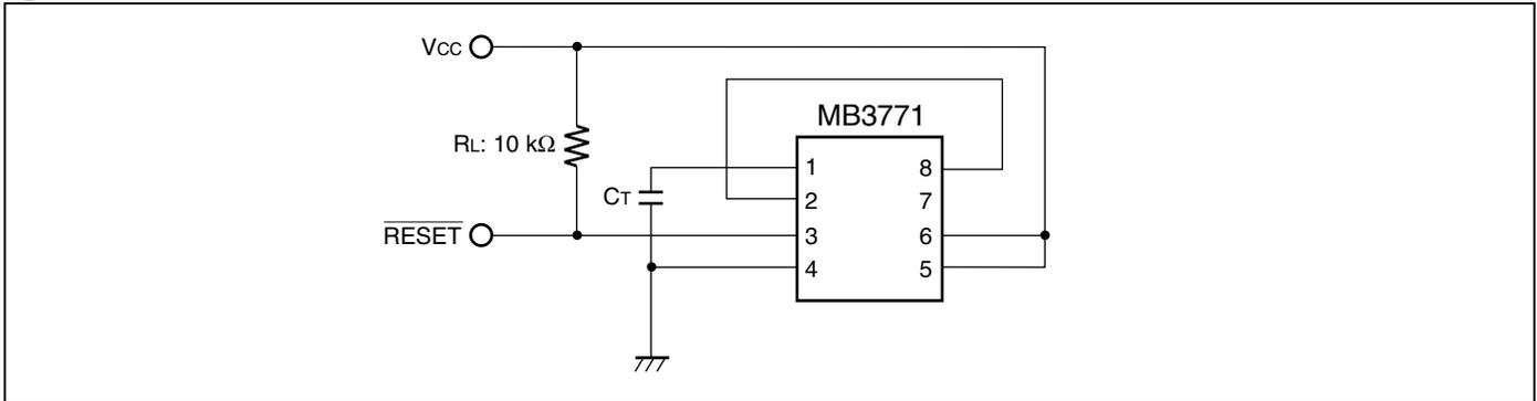
**8.8 Supply Voltage Monitoring with Delayed Trigger**
