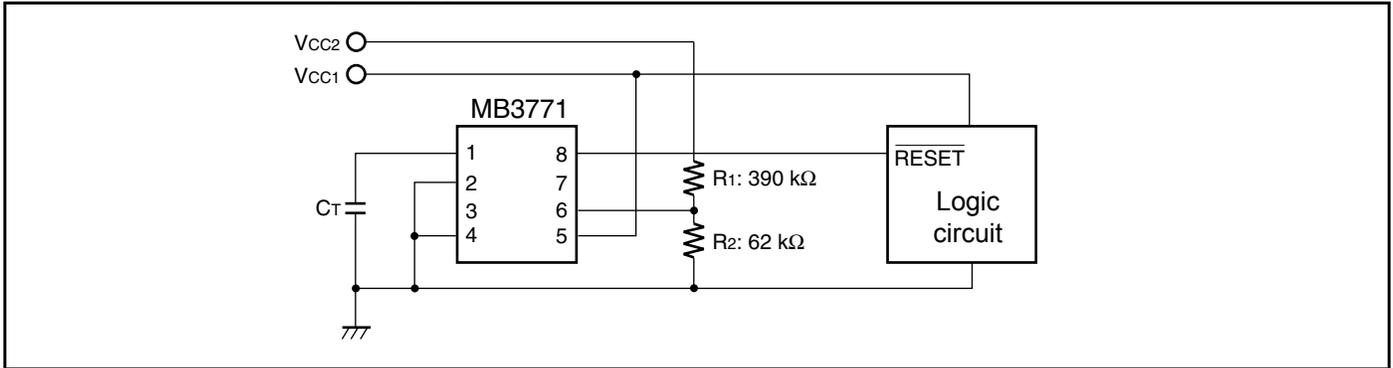
**8.5 5 V and 12 V Power Supply Monitor ( $\overline{\text{RESET}}$  signal is generated by 5 V,  $V_{CC1} = 5\text{ V}$ ,  $V_{CC2} = 12\text{ V}$ )**
