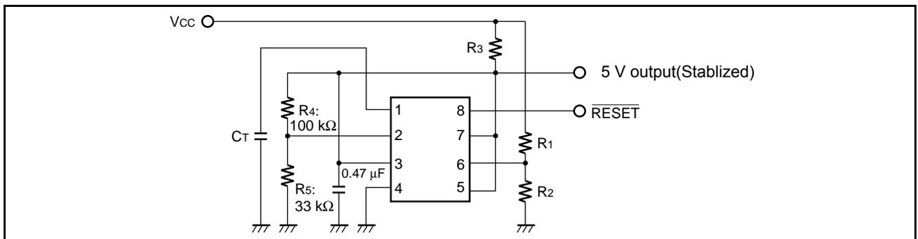
**8.4 5 V and 12 V Power Supply Monitor (2 types of power supply monitor  $V_{CC1} = 5\text{ V}$ ,  $V_{CC2} = 12\text{ V}$ )**
