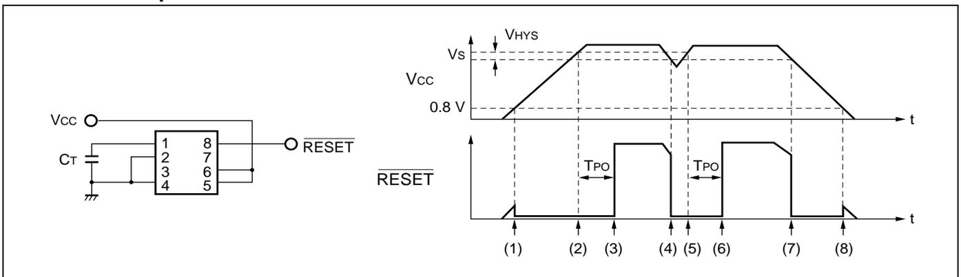
1. When  $V_{CC}$  rises to about 0.8V,  $\overline{RESET}$  goes low.
