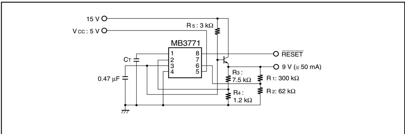
**8.10.2 5 V Reference Voltage Generation and 5V Monitoring (No.1)**
