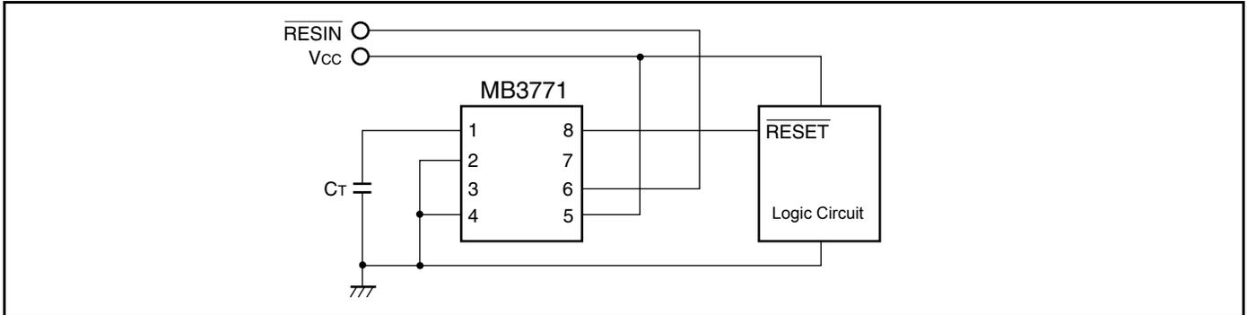
**8.7 5 V Power Supply Monitor with Non-inverted  $\overline{\text{RESET}}$**
