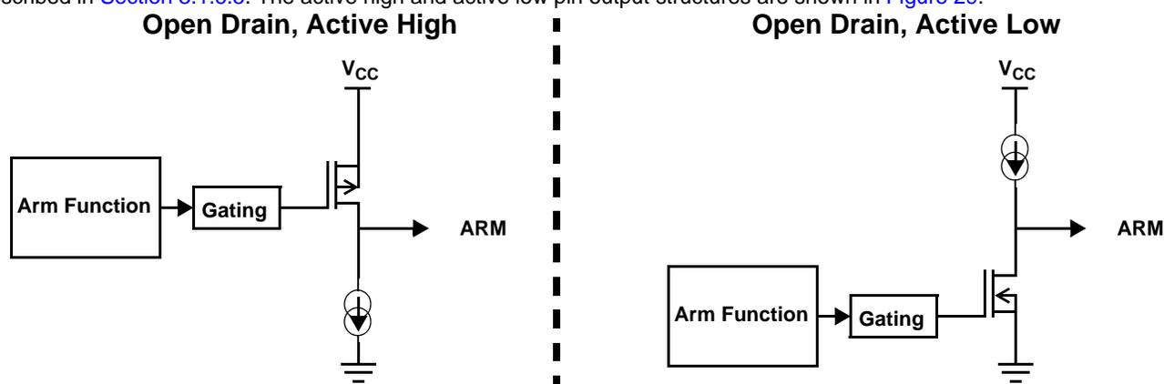
Figure 29. Arming Function - Pin Output Structure
