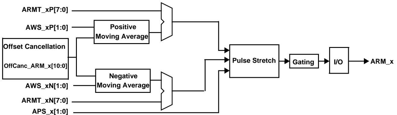
Figure 24. Arming Function Block Diagram - Moving Average Mode
