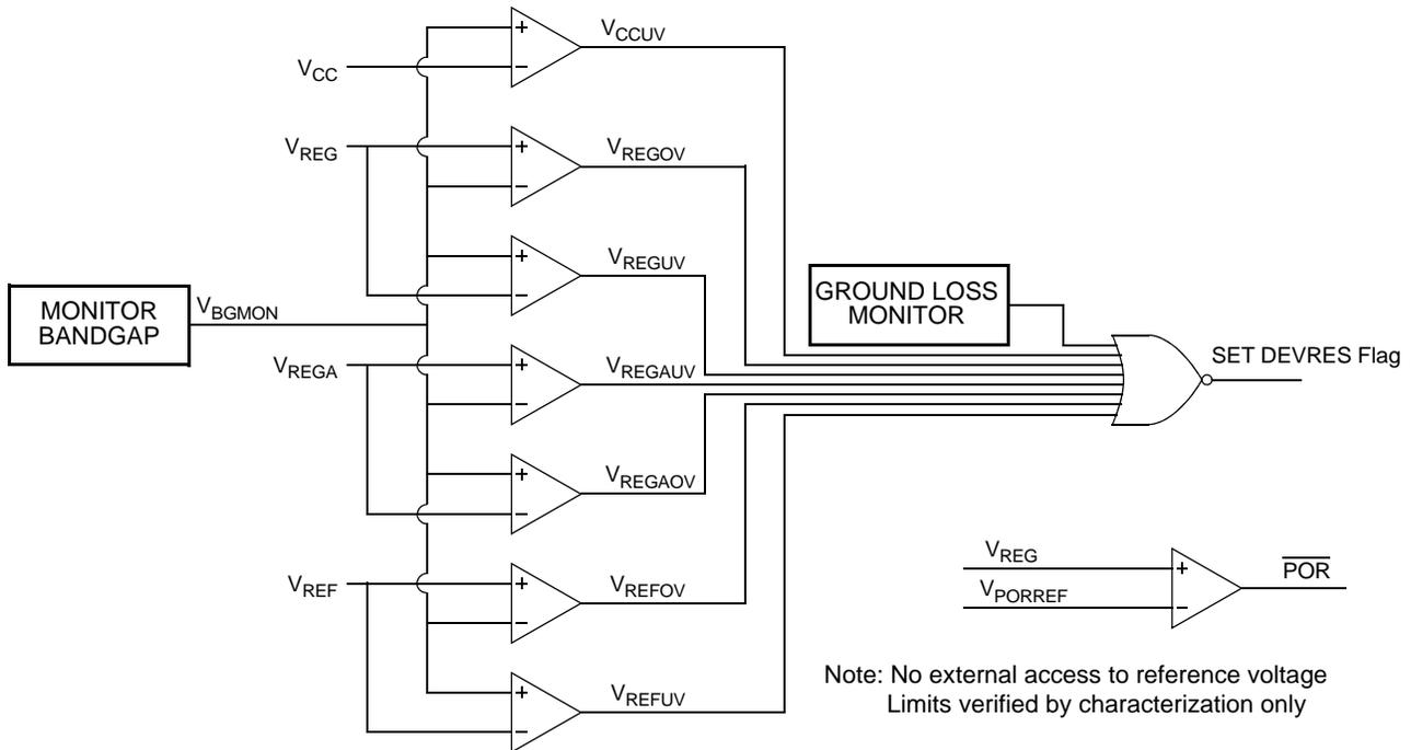
Figure 9. Voltage Monitoring
