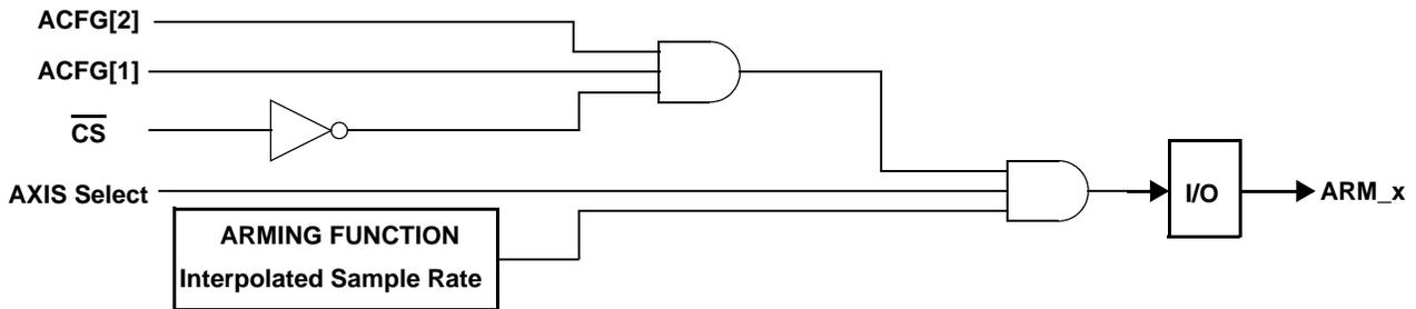
Figure 27. Arming Function Block Diagram - Unfiltered Mode
