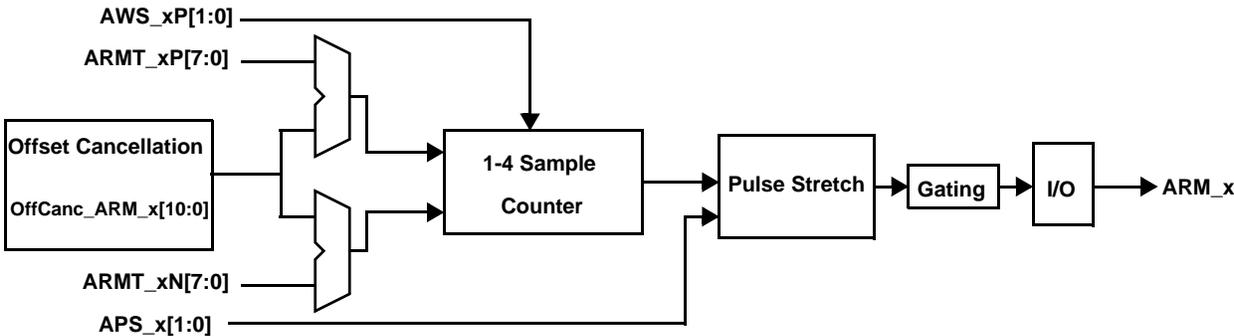
Figure 25. Arming Function Block Diagram - Count Mode
