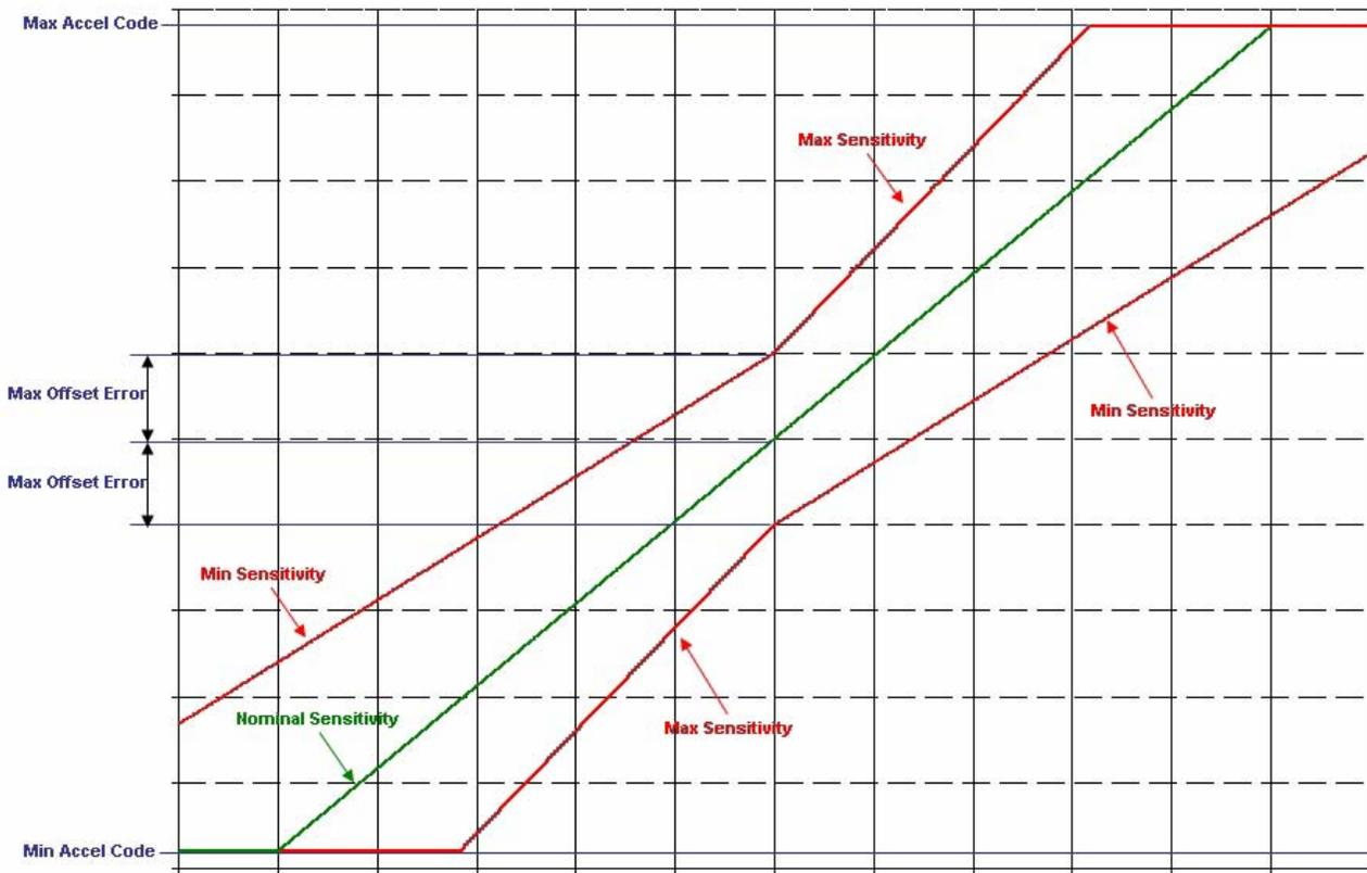
Figure 36. Acceleration Data Output Vs. Acceleration Input
