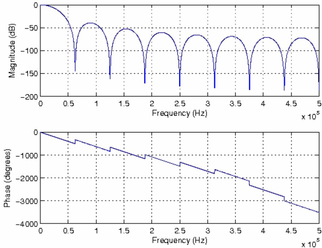
Figure 14. Sinc Filter Response,  $t_S = 8 \mu s$
