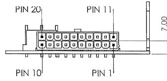
**NVM175 Vertical Connector With Optional Case And Cover (-C Option)**
