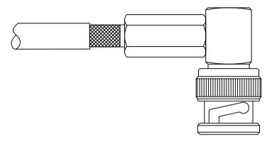
4) Firmly push the cable as far forward as possible and screw the connector hex back end onto the cable in a clockwise direction until it stops.
