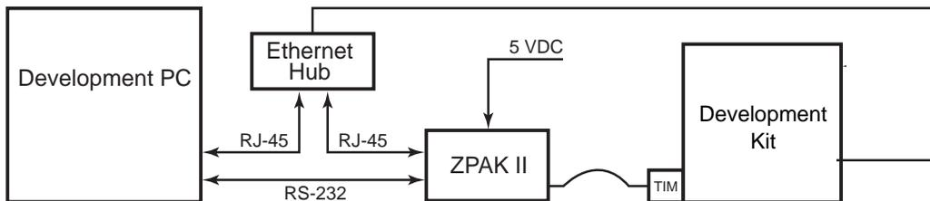
**Figure 1. Hardware Setup using an Ethernet Hub**
