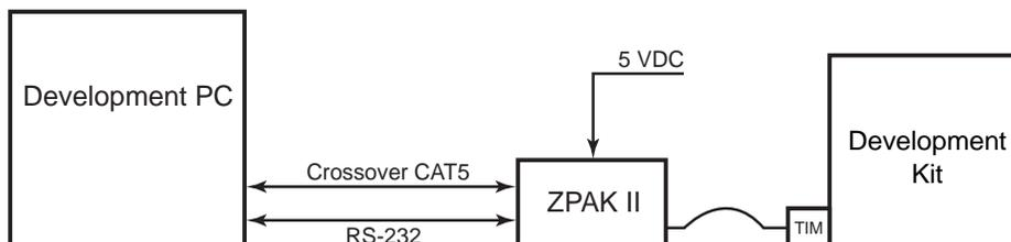
**Figure 2. Hardware Setup using a Crossover Ethernet Cable**
