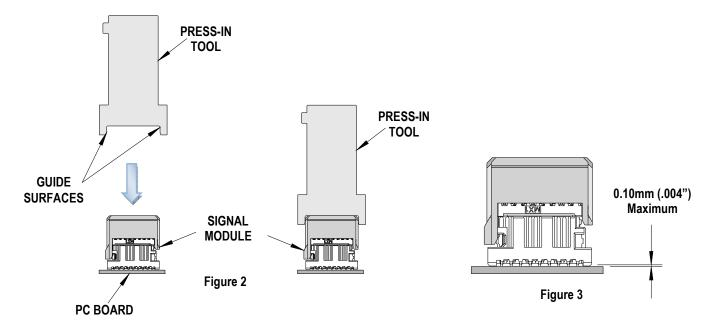
3. Using the application tool and an appropriate press, seat the Signal module until there is less than 0.10mm (.004 in.) clearance between the bottom of the plastic housing and the surface of the PCB. See Figure 3.
