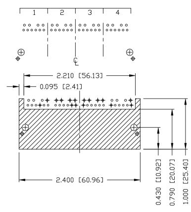
THE SHADED AREA ON THE CUSTOMER BOARD ARE RECOMMENDED TO BE CLEAR OFF ANY VIA HOLE OR COMPONENT PAD.
