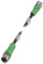
Sensor/Actuator cable, 8-position, PUR halogen-free, black-gray RAL 7021, Plug straight M12, A-coded, on Socket straight M12, A-coded, Cable length: 20 m
