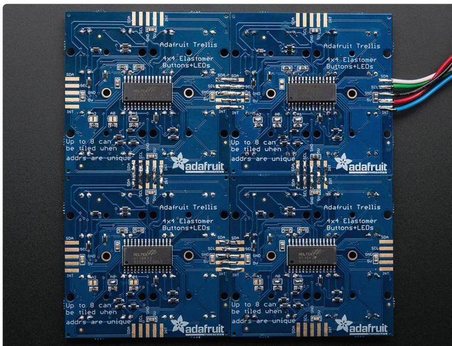
Each LED is multiplexed with a constant-current driver, so you can mix and match any colors you like. You don't need it to be all blue, all red, etc. Mix it up! Any 3mm LED can be used, although we find that diffused LEDs with 250mcd+ brightness look best.
