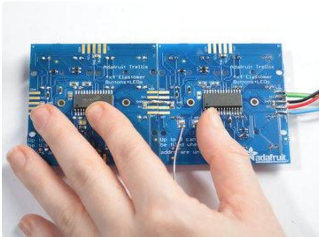
For a more robust connection, use a small bare wire across the pads instead of just solder. The legs trimmed off the LEDs are perfect for this!
