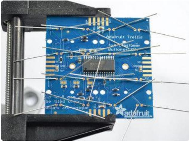
You can do one LED at a time, or all at once, its up to you and how experienced you are in soldering LEDs.
