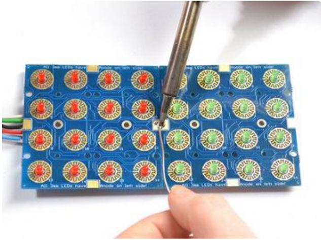
You can add a little more mechanical stability by soldering the large front tabs as well
