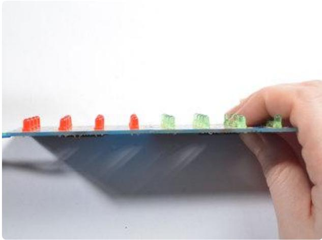
Check that the panels are aligned by looking from the side, gently bend/reheat until they are nice and straight
