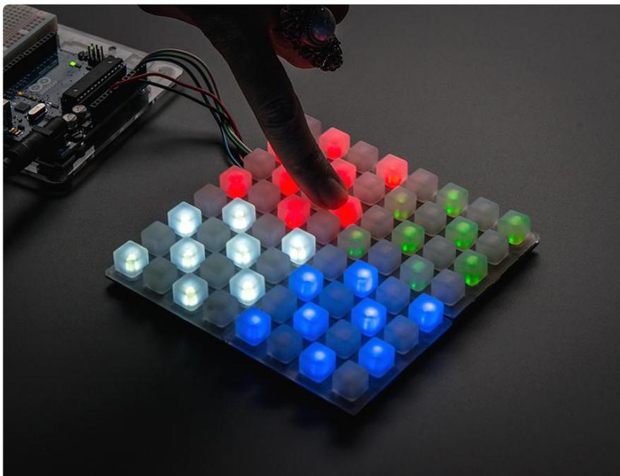
You can tile up to eight Trellis PCBs on a single 2-wire I2C bus. This allows you to easily build up to 8x16 or 4x32 panels which can be lots of fun!
