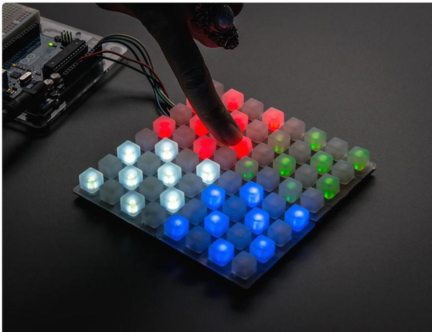
Trellis is an open source backlight keypad driver system. It is easy to use, works with any 3mm LEDs and eight tiles can be tiled together on a shared I2C bus.
