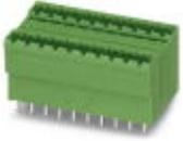
Header, Nominal current: 10 A, Rated voltage (III/2): 320 V, Number of positions: 12, Pitch: 5 mm, Color: green, Contact surface: Tin, Assembly: Soldering, In combination with MVSTB or FKCV plug components, both an MVSTBW (or FKCVW) and an MVSTBR plug (or FKCVR) must be used. Combination with TMSTBP plug components is not possible!
