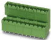
Header, Nominal current: 10 A, Rated voltage (III/2): 320 V, Number of positions: 12, Pitch: 5 mm, Color: green, Contact surface: Tin, Assembly: Soldering, The article can be aligned to create different nos. of positions! In combination with MVSTB or FKCV plug components, both an MVSTBW (or FKCVW) and an MVSTBR plug (or FKCVR) must be used. Combination with TMSTBP plug components is not possible!
