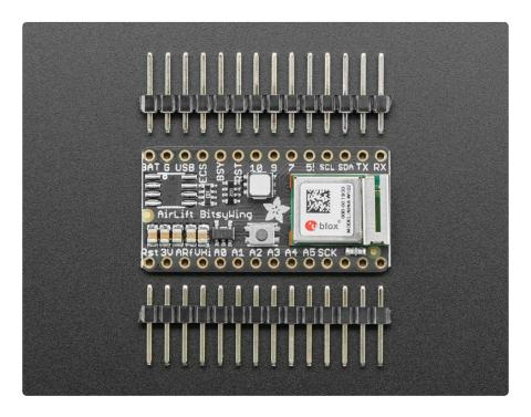
We placed an ESP32 module on a BitsyWing with a tri-state chip for MOSI so you can share the SPI bus. The add on comes fully assembled and tested, pre-programmed with ESP32 SPI WiFi co-processor firmware that you can use in CircuitPython to use this into WiFi co-processor over SPI + 2 pins (). We also toss in some header so you can solder it in though you'll need stacking headers for your ItsyBitsy to put the add-on on top.
