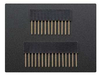
To stack the Airlift Add-on on top of the ItsyBitsy, you'll need stacking headers for the ItsyBitsy. For now you'll need to cut down a set of Feather Stacking Headers () to fit the ItsyBitsy however we will have headers with the correctly length soon!
