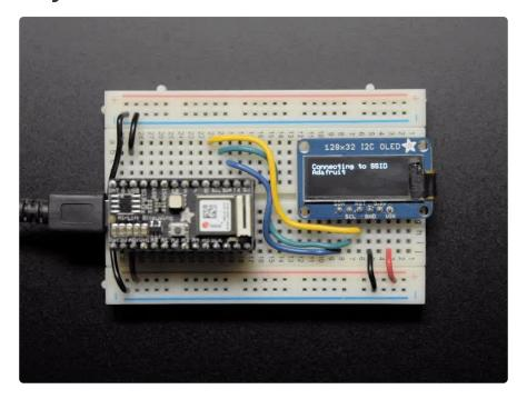
The antenna on the new, smaller ESP32 module is very delicate! Avoid touching it and grab the add-on by the long sides to avoid smushing the antenna
