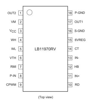
PGND: Motor system GND SGND: Control system GND
