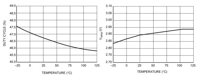
Figure 15. NCP1216A Max Duty-Cycle vs. Temperature
