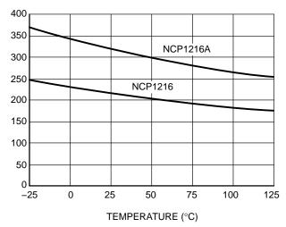
Figure 9. VCC<sub>latch</sub> vs. Temperature
