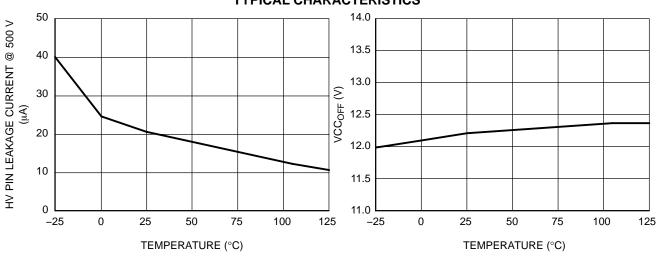
Figure 3. High Voltage Pin Leakage Current vs.
