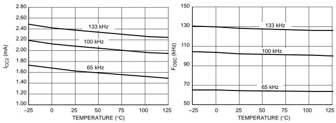
Figure 7. I<sub>CC2</sub> vs. Temperature
