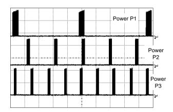
Figure 22. Output Pulses at Various Power Levels (X = 5 μs/div) P1 < P2 < P3
