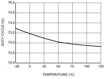
Figure 13. V<sub>skip</sub> vs. Temperature
