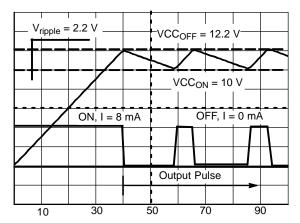
Figure 18. The Charge/Discharge Cycle Over a 10  $\mu$ F V<sub>CC</sub> Capacitor
