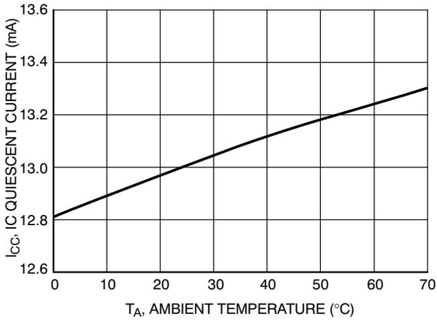
Figure 4. IC Quiescent Current vs. Ambient Temperature
