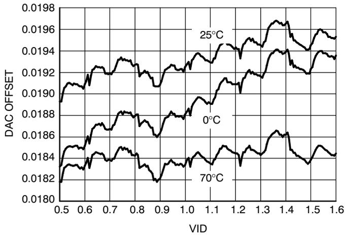
Figure 6. Typical DAC Voltage Offset vs. Temperature
