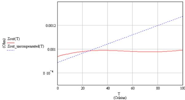
**Figure 19. Uncompensated and Compensated Output Impedance vs. Temperature**
