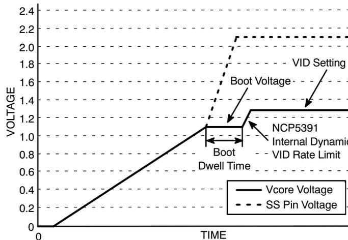
Figure 7. Typical VR11 Soft-Start Sequence to Vcore = 1.3 V
