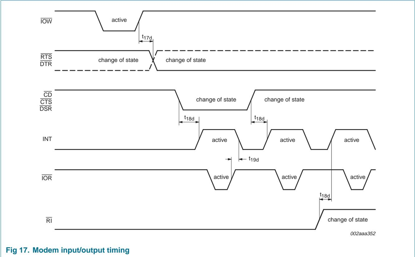
Fig 17. Modem input/output timing
