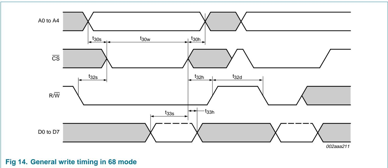
Fig 14. General write timing in 68 mode
