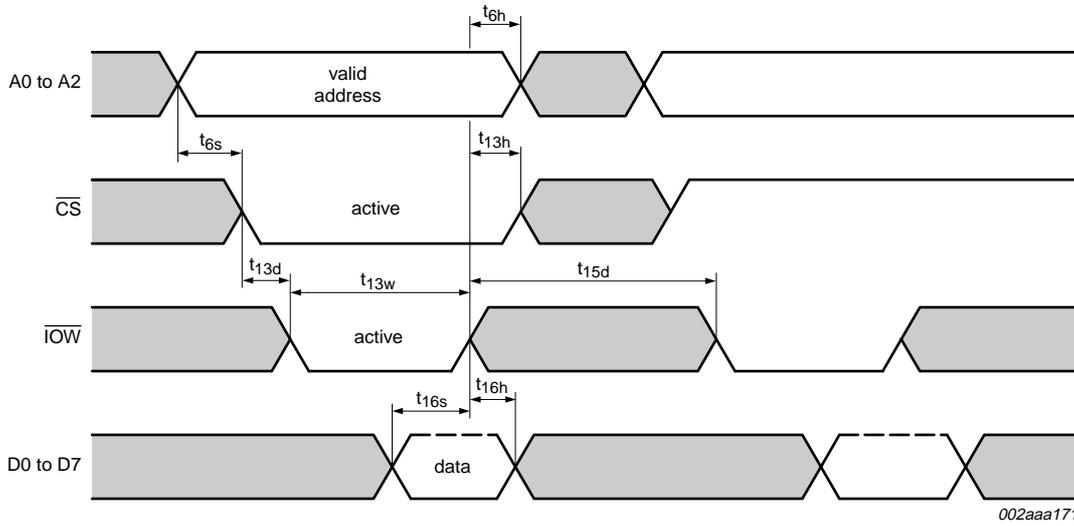
Fig 15. General write timing in 16 mode
