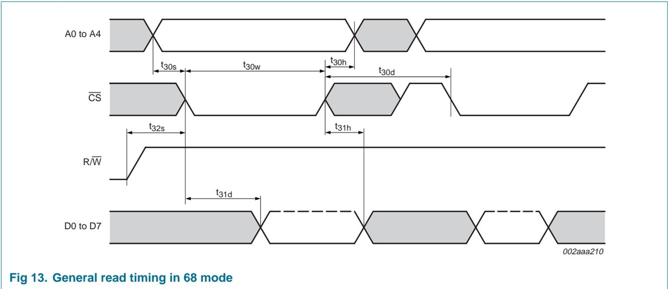
Fig 13. General read timing in 68 mode
