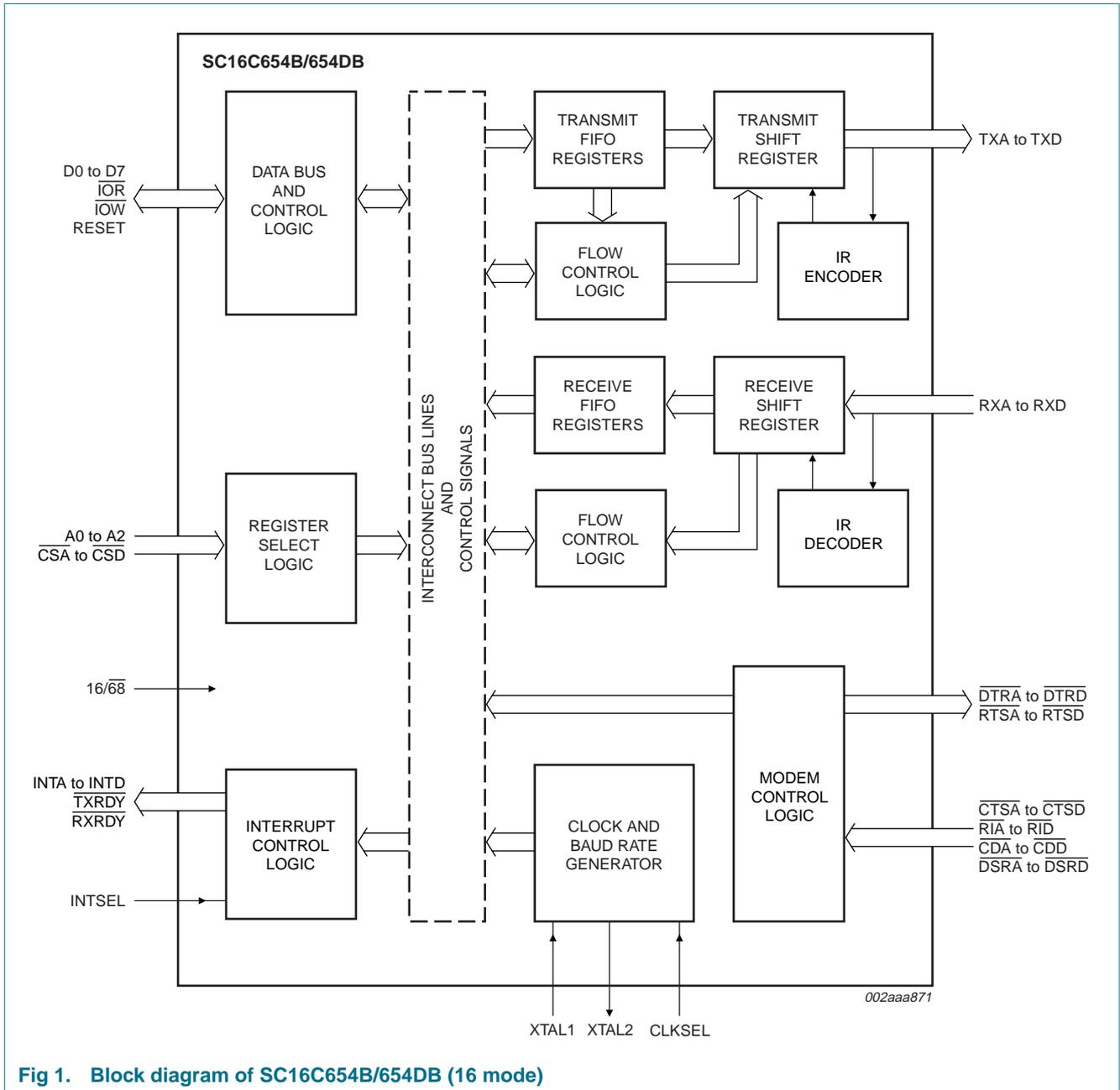
Fig 1. Block diagram of SC16C654B/654DB (16 mode)
