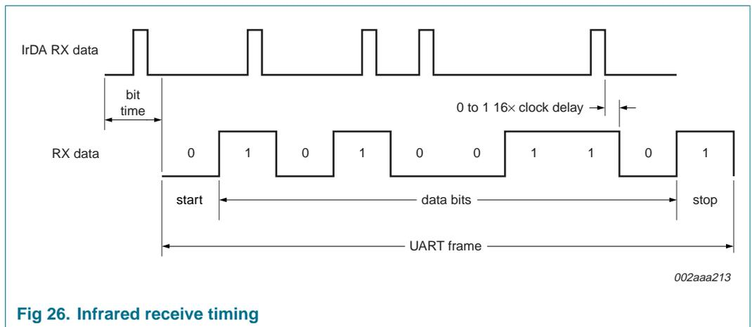
Fig 26. Infrared receive timing
