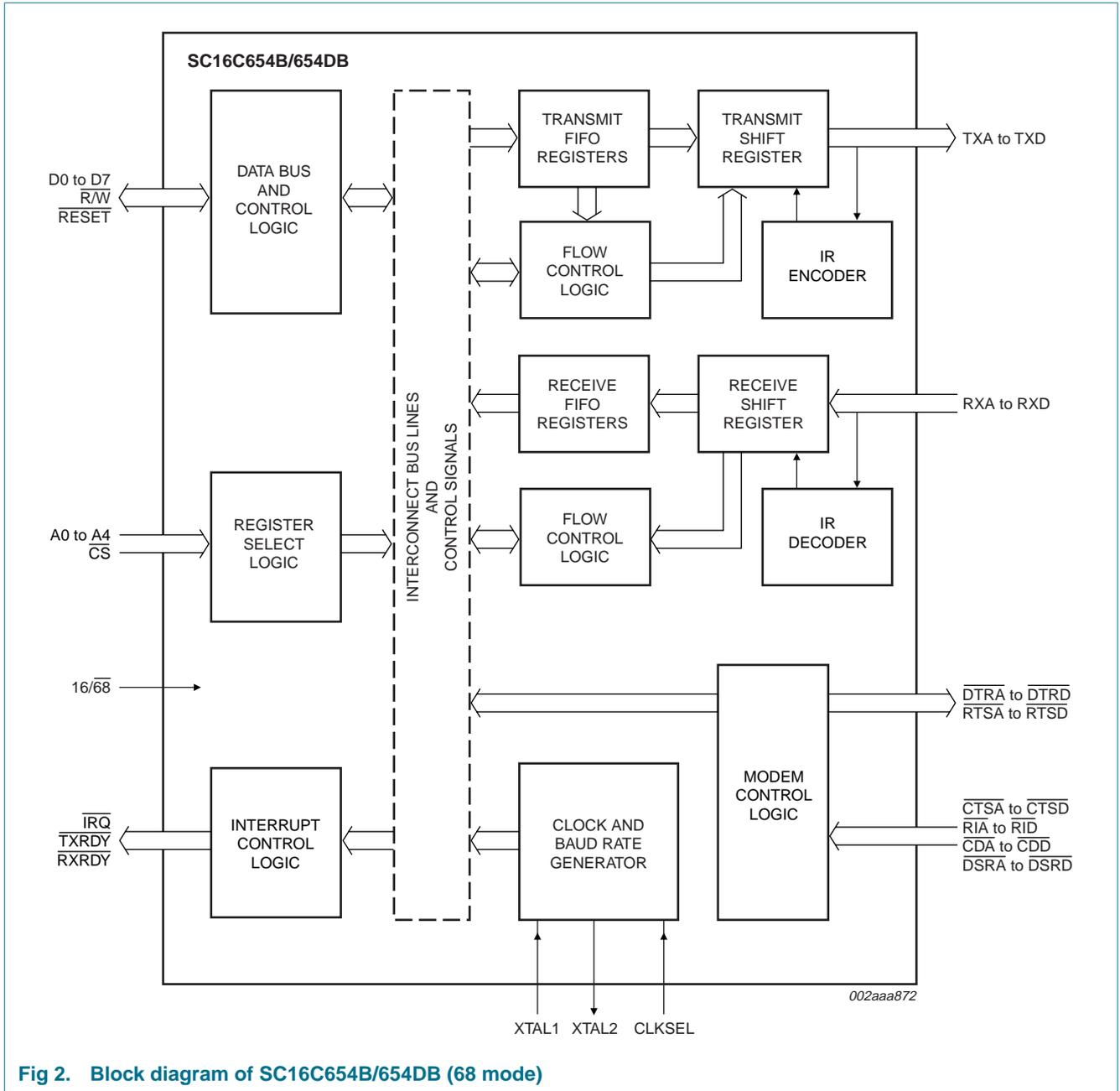
Fig 2. Block diagram of SC16C654B/654DB (68 mode)
