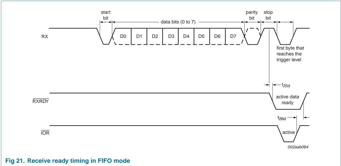
Fig 21. Receive ready timing in FIFO mode
