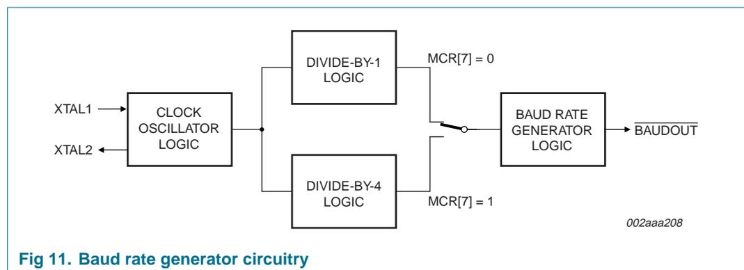
**Fig 11. Baud rate generator circuitry**
