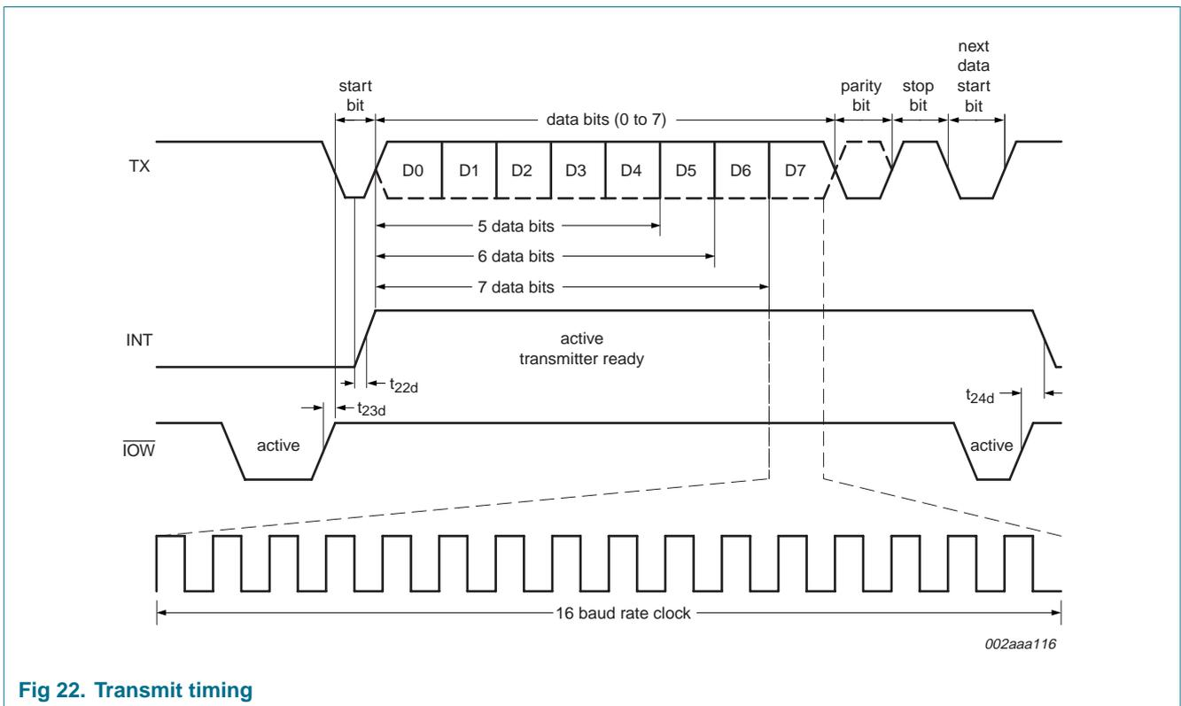
Fig 22. Transmit timing
