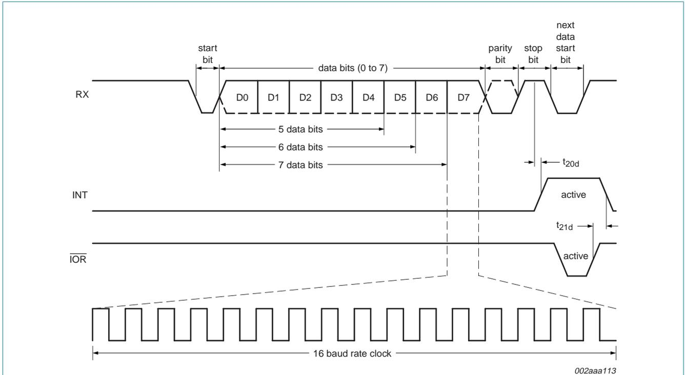
Fig 19. Receive timing
