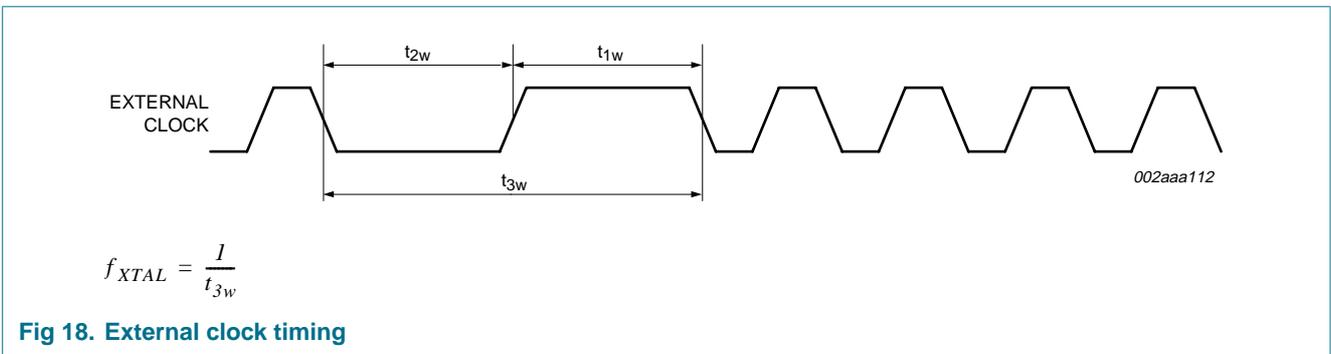
Fig 18. External clock timing
