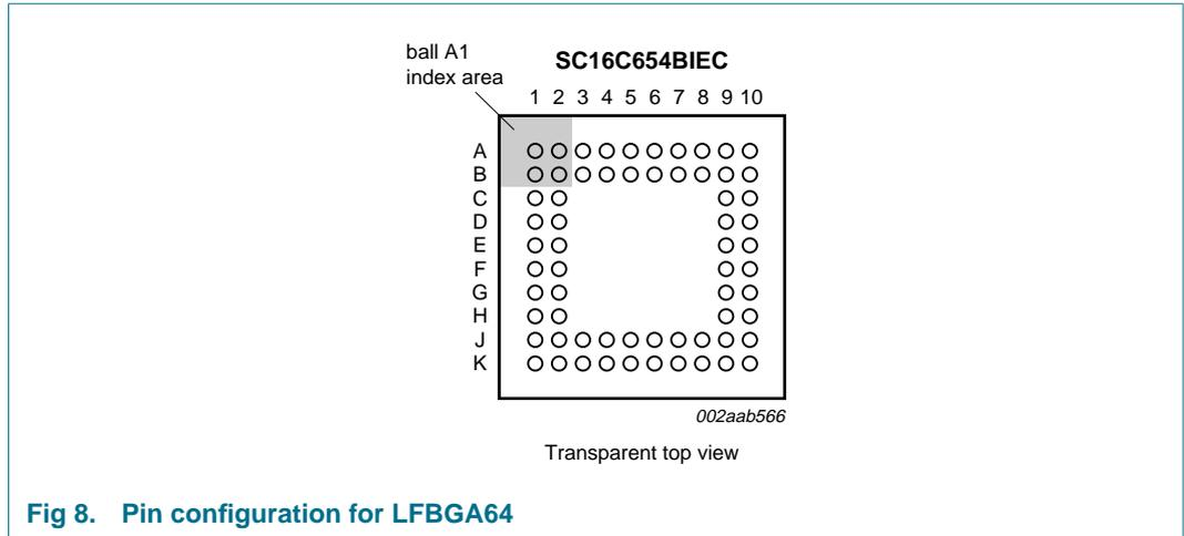
Fig 8. Pin configuration for LFBGA64
