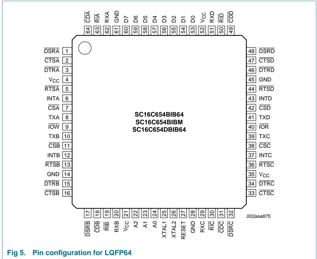
Fig 5. Pin configuration for LQFP64
