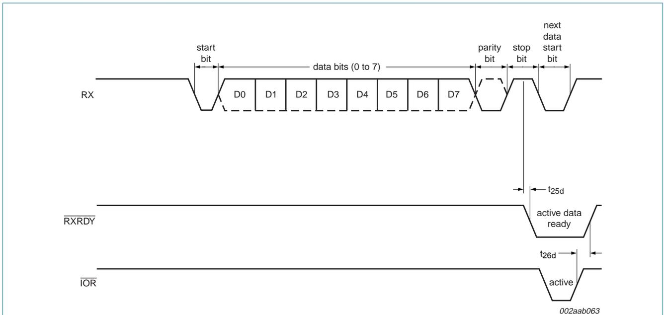
Fig 20. Receive ready timing in non-FIFO mode
