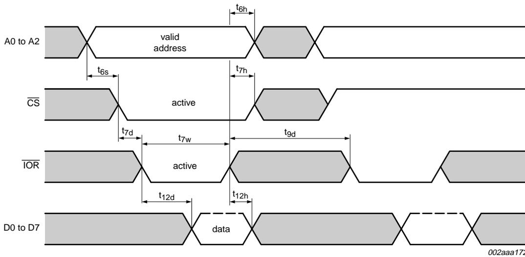
Fig 16. General read timing in 16 mode
