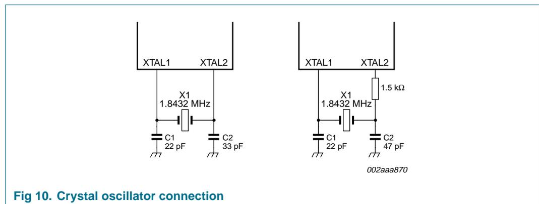
Fig 10. Crystal oscillator connection
