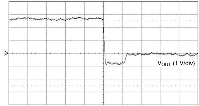
$V_{IN} = 2.8\text{ V}$ ,  $R_{LOAD} = 18\ \Omega$ ,  $L_{LOAD} = 80\ \mu\text{H}$
