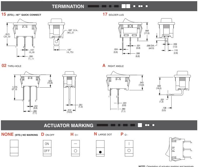
NOTE: Orientation of actuator marking and terminals.
