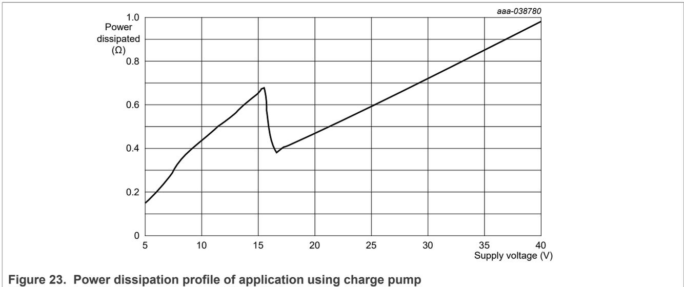
Figure 23. Power dissipation profile of application using charge pump
