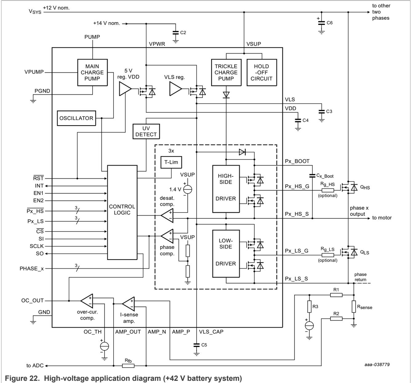
Figure 22. High-voltage application diagram (+42 V battery system)
