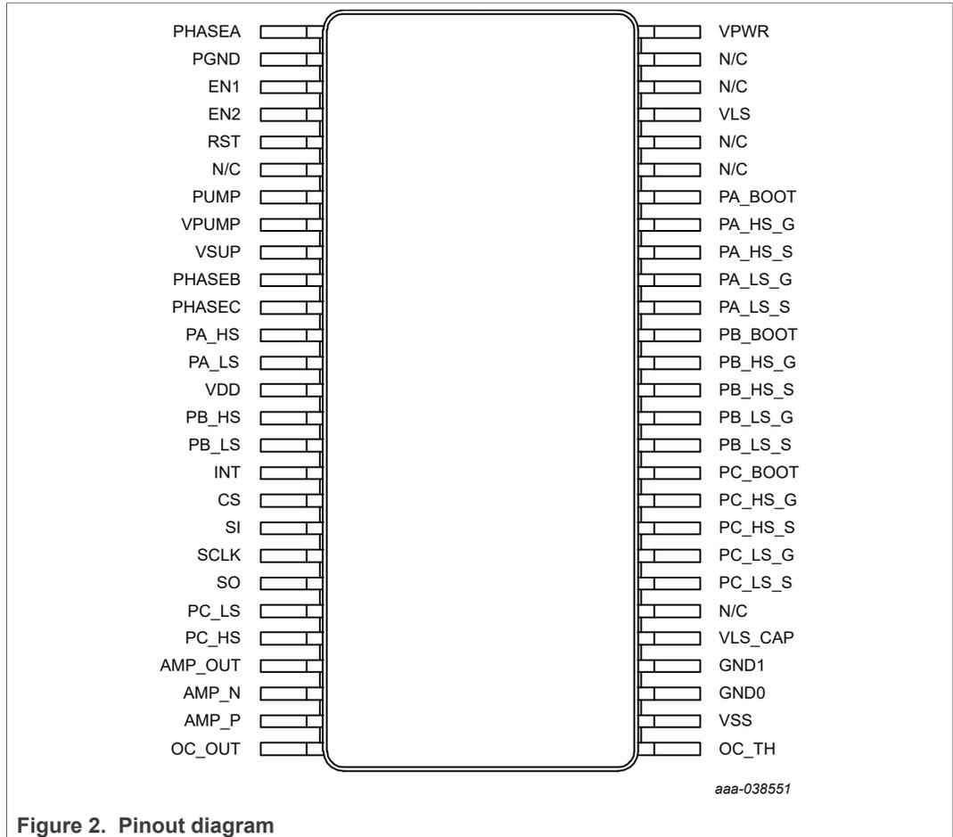
Figure 2. Pinout diagram
