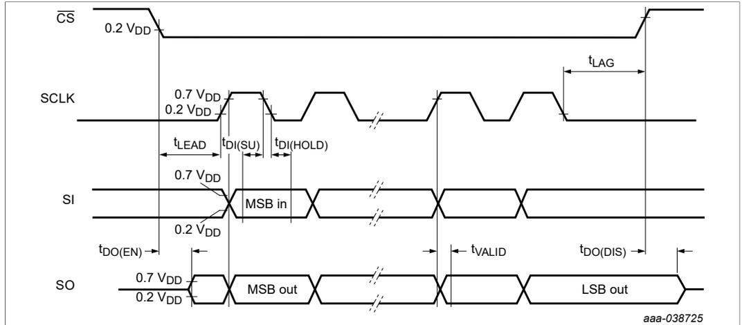
Figure 3. SPI interface timing
