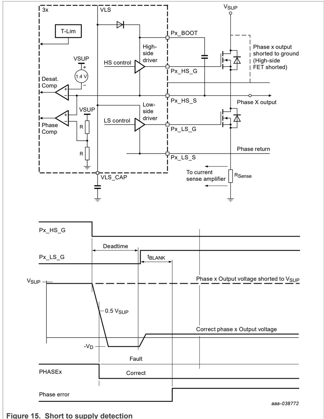
Figure 15. Short to supply detection
