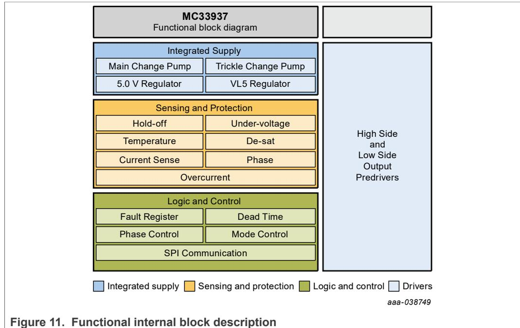
Figure 11. Functional internal block description
