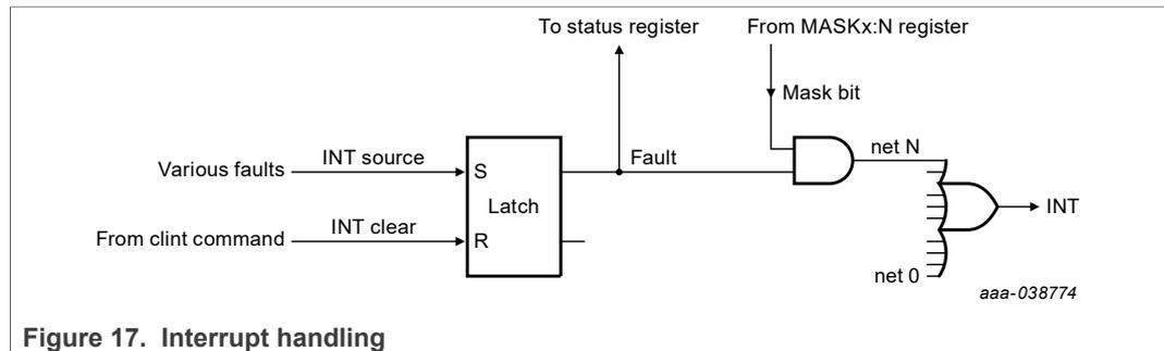
Figure 17. Interrupt handling
