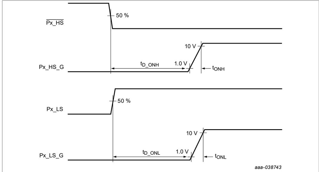
Figure 6. Driver turn-on time and turn-on delay
