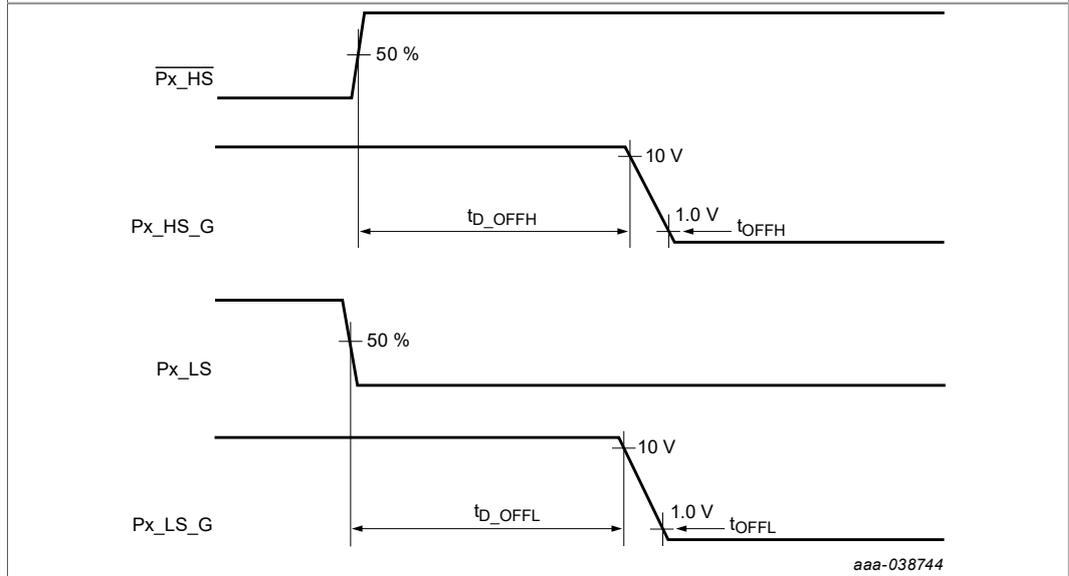
Figure 7. Driver turn-off time and turn-off delay
