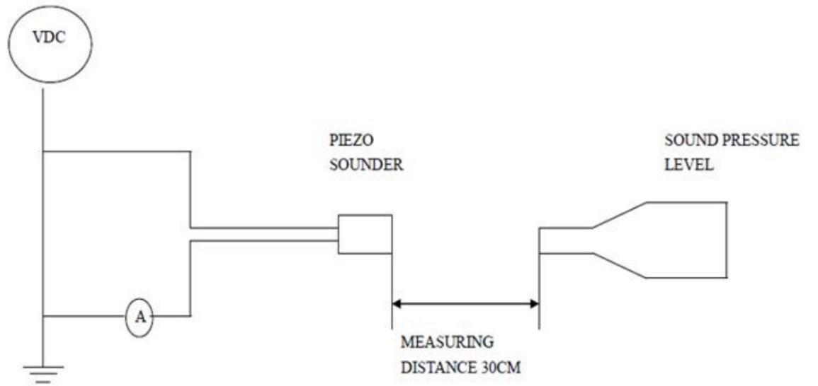
MIC: S.P.L meter TES1351B or equivalent
