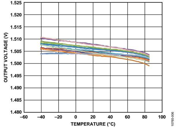
Figure 6. X-Axis Zero g Offset vs. Temperature,  $V_s = 3\text{ V}$
