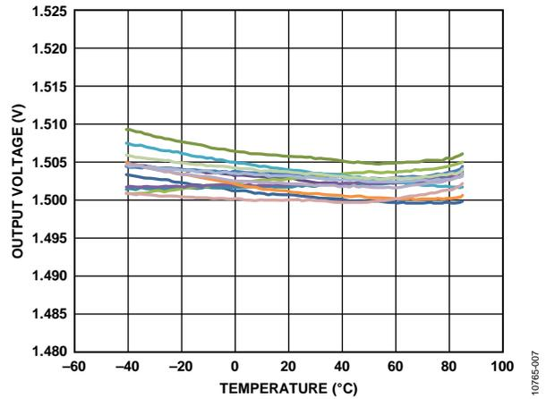
Figure 7. Y-Axis Zero g Offset vs. Temperature,  $V_s = 3\text{ V}$
