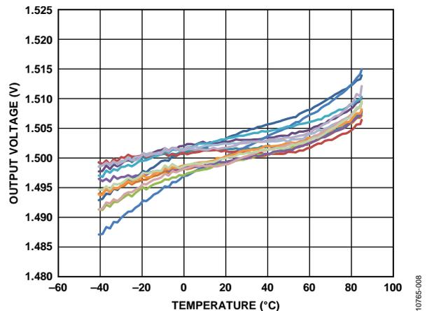
Figure 8. Z-Axis Zero g Offset vs. Temperature,  $V_s = 3\text{ V}$
