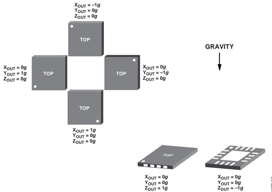
Figure 15. Output Response vs. Orientation to Gravity
