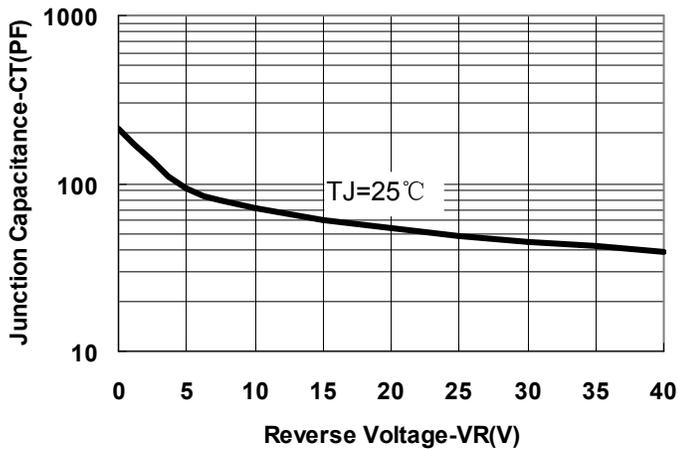
Fig.1-Typical Junction Capacitance
