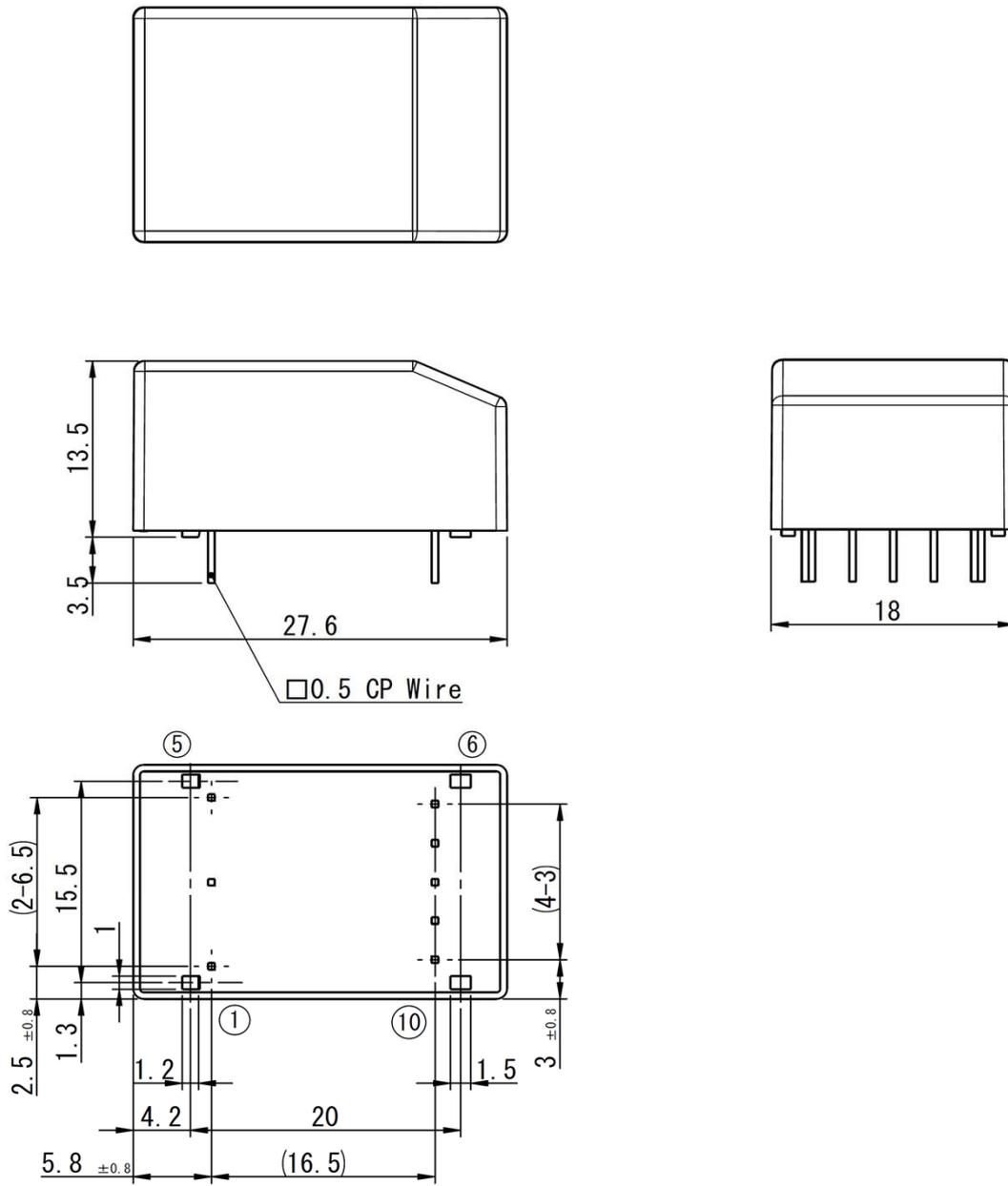
Note : 1.The dimensional tolerance without directions is  $\pm 0.5\text{mm}$ .
