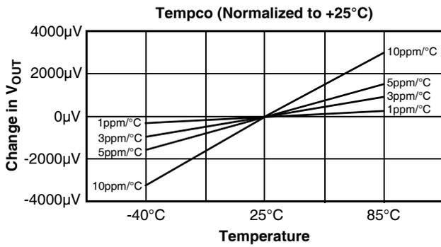
The tempco curve for the X60008 devices is generally flat (within 0.5ppm/°C typically) over the industrial temperature range (-40 to 85°C) with some inflection at the extreme temperatures. The combination of very low tempco performance a predictable tempco slope is unique to the X60008 due to its floating gate technology. This behavior is much easier to consider when designing data conversion systems or control systems that must operate over a range of temperatures.
