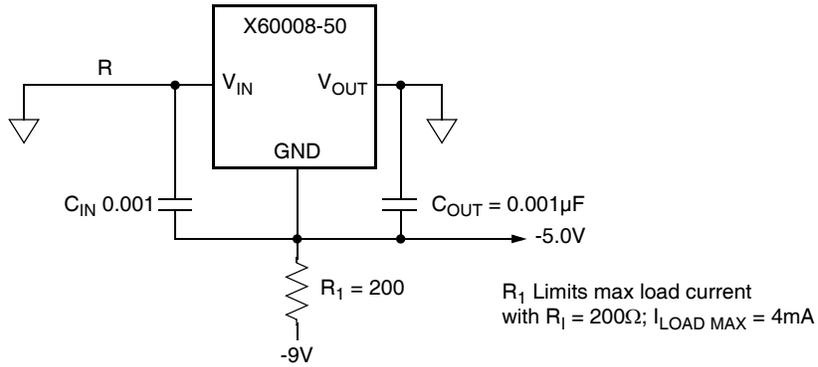
5V Full Scale Low-Drift 10-bit Adjustable Voltage Source
