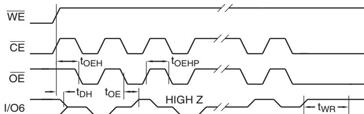
Notes: 1. Toggling either  $\overline{OE}$  or  $\overline{CE}$  or both  $\overline{OE}$  and  $\overline{CE}$  will operate toggle bit. The  $t_{OEHP}$  specification must be met by the toggling input(s).
