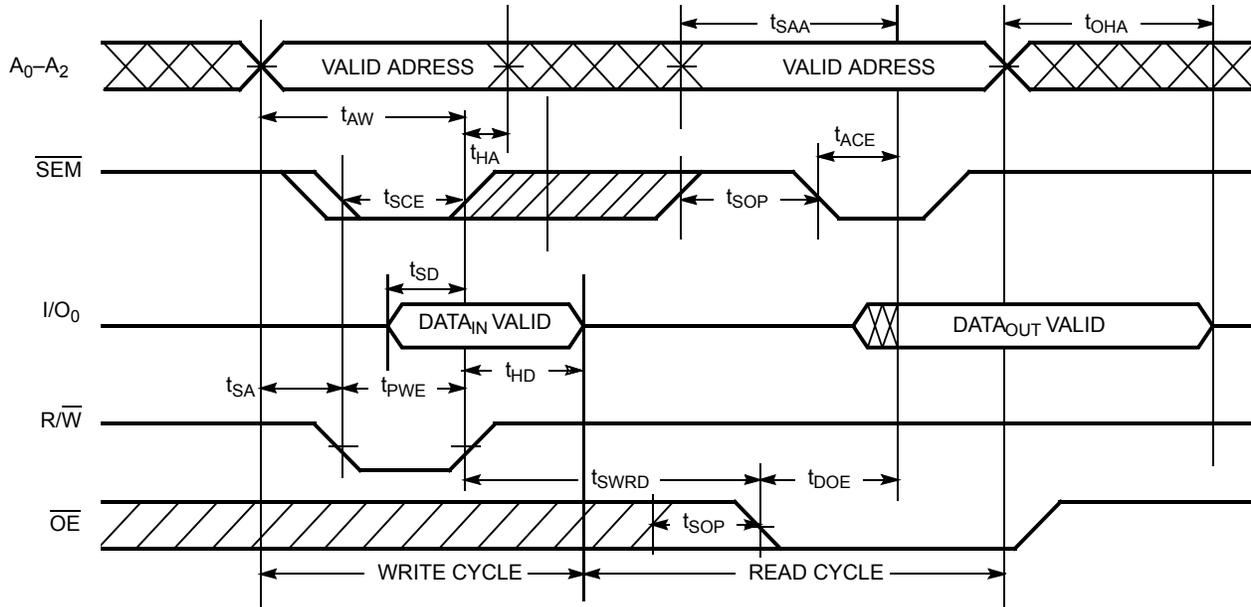
**Figure 10. Timing Diagram of Semaphore Contention [50, 51, 52]**
