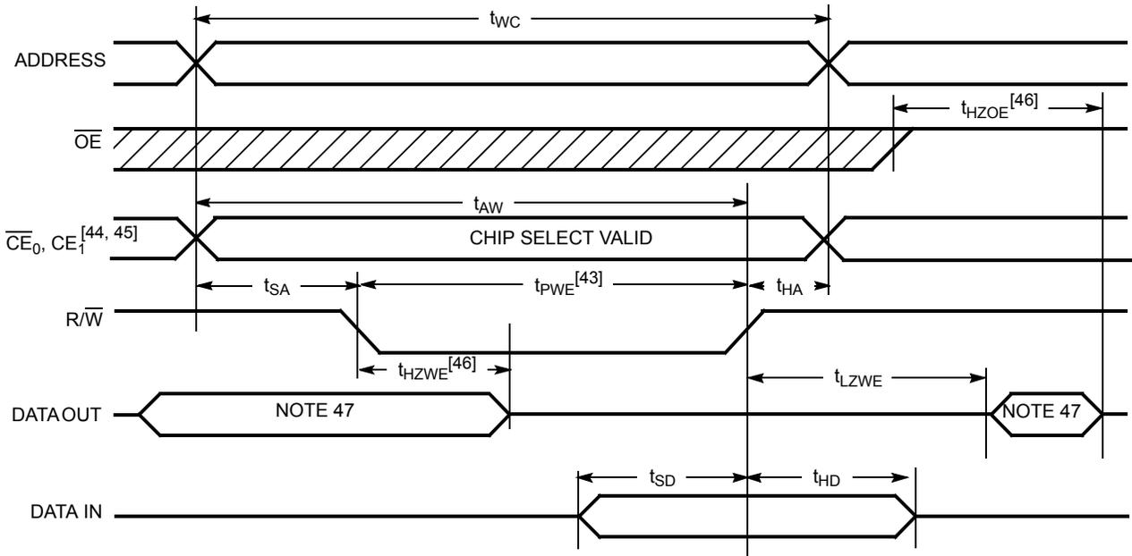
Figure 8. Write Cycle No. 2 (CE Controlled Timing) [40, 41, 42, 48]
