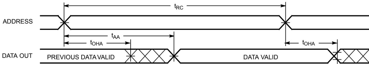
Figure 5. Read Cycle No. 2 (Either Port  $\overline{CE}/\overline{OE}$  Access) [35, 38, 39]
