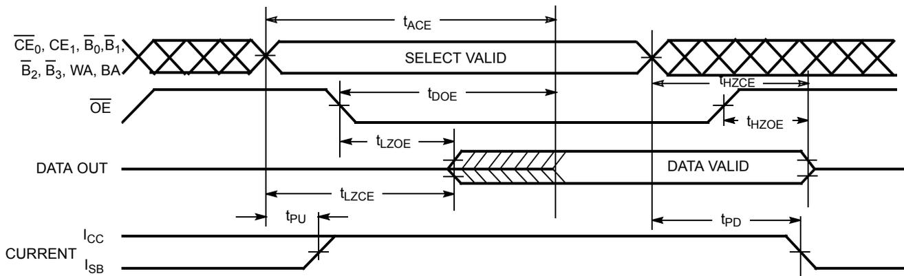
Figure 6. Read Cycle No. 3 (Either Port) [35, 37, 38, 39]
