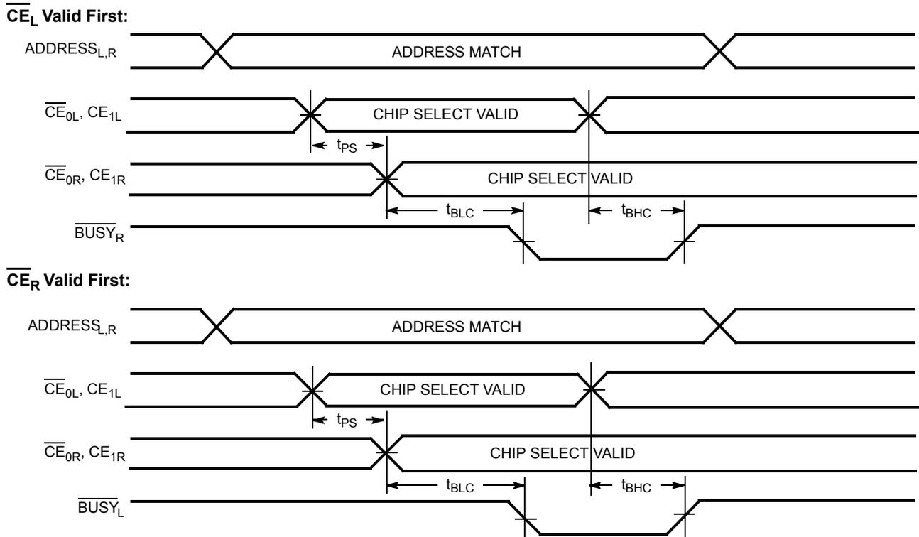
Figure 14. Busy Timing Diagram No. 2 (Address Arbitration) [54]
