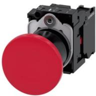
Mushroom pushbutton, 22 mm, round, plastic, red, 40mm, latching, pull-tounlatch mechanism, with holder, 1 NC, screw terminal, with laser labeling, upper case and lower case, always upper case at beginning of line
