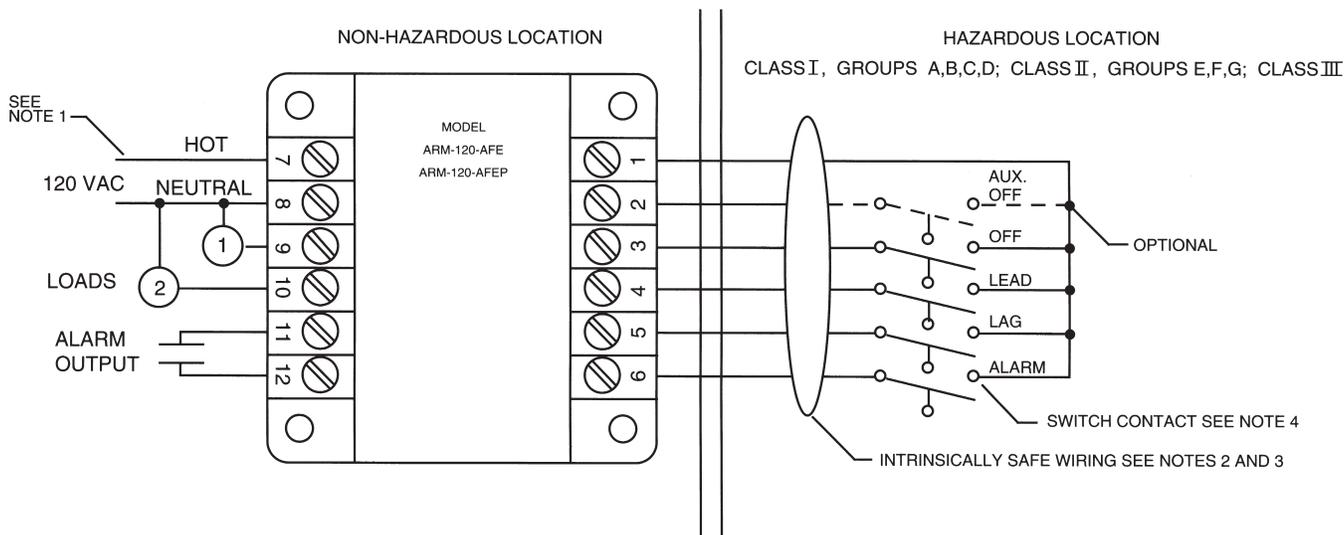
1. To maintain intrinsic safety, connect the Controller's Earth Ground Terminal 8 to the earth ground of the AC Power Supply feeder. The resistance between the Controller's Earth Ground Terminal and Earth Ground shall be less than 1 ohm.
