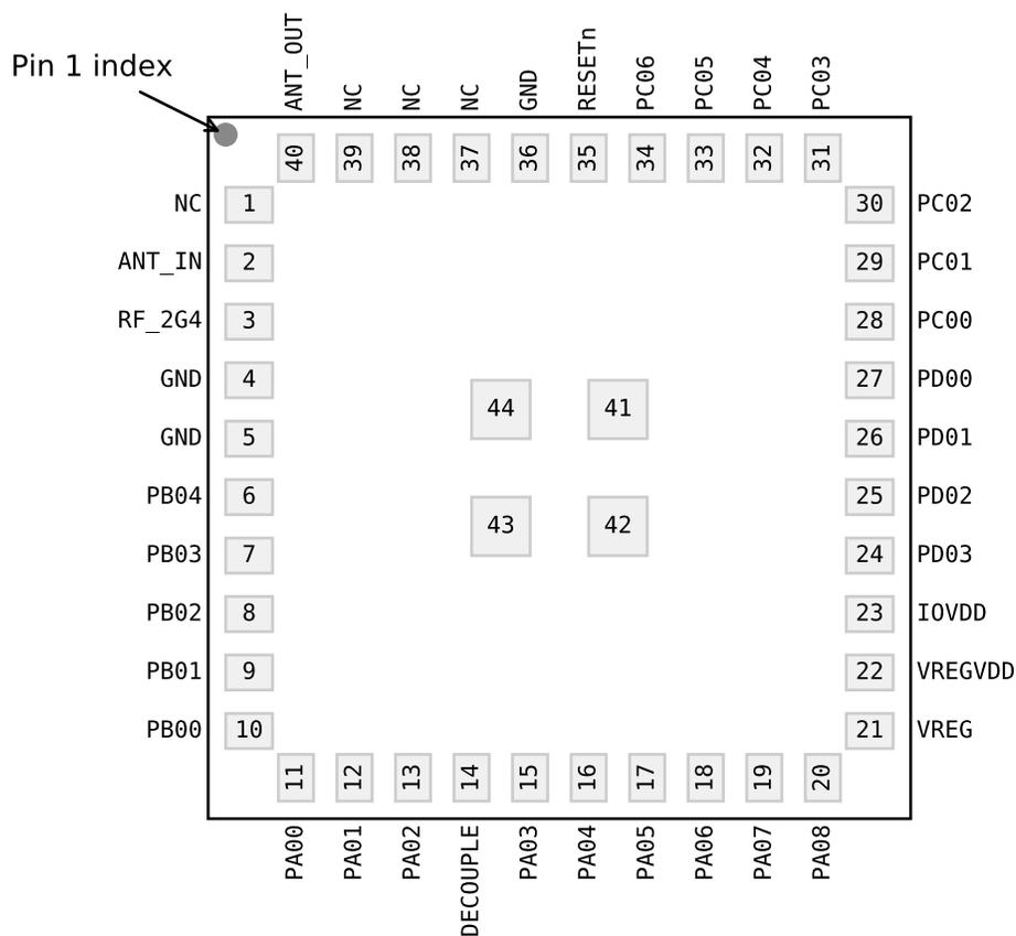
**Figure 6.1. 44-Pin SiP Module Device Pinout**
