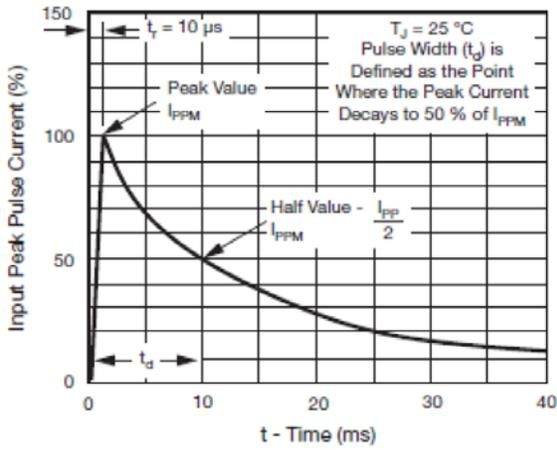
Fig. 3 - Pulse Waveform
