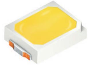
The DURIS® E 2 combines high efficacy and a wide beam angle into a compact format (2.0 mm x 1.6 mm). It is ideal for lighting applications requiring a homogeneous distributed light source, like tube lighting, panel lighting, troffer.
