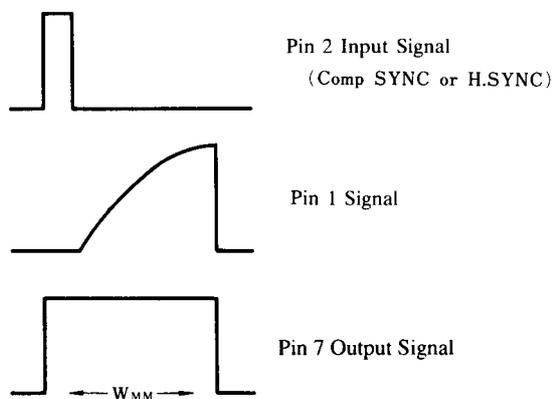
Adjust Pin 7 DC Voltage to 2V (at  $V^+=5V$ ) by varying Pin 1 outer resistor, and test Pin7 output pulse width after taking off Pin7 outer capacitor.
