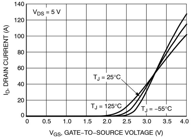
Figure 2. Transfer Characteristics
