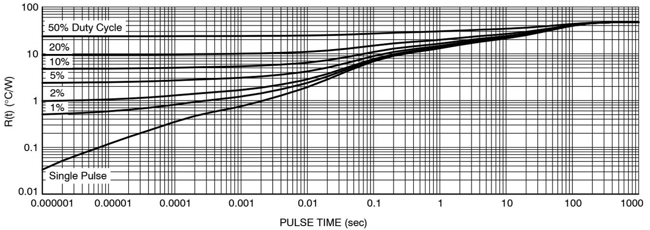
Figure 13. Thermal Characteristics
