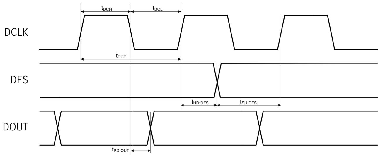
**Figure 6. Digital Audio Interface Timing Parameters, I<sup>2</sup>S Mode**
