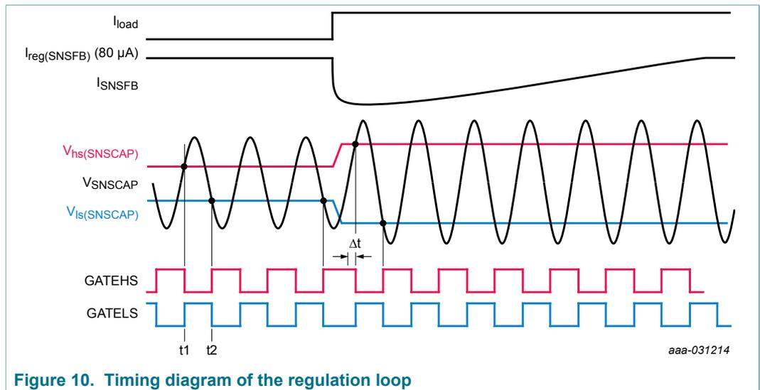
Figure 10. Timing diagram of the regulation loop
