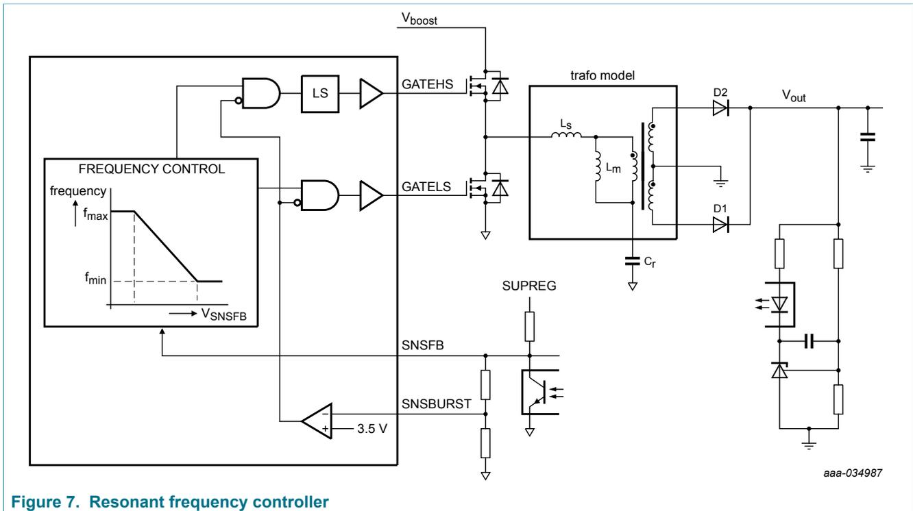
Figure 7. Resonant frequency controller
