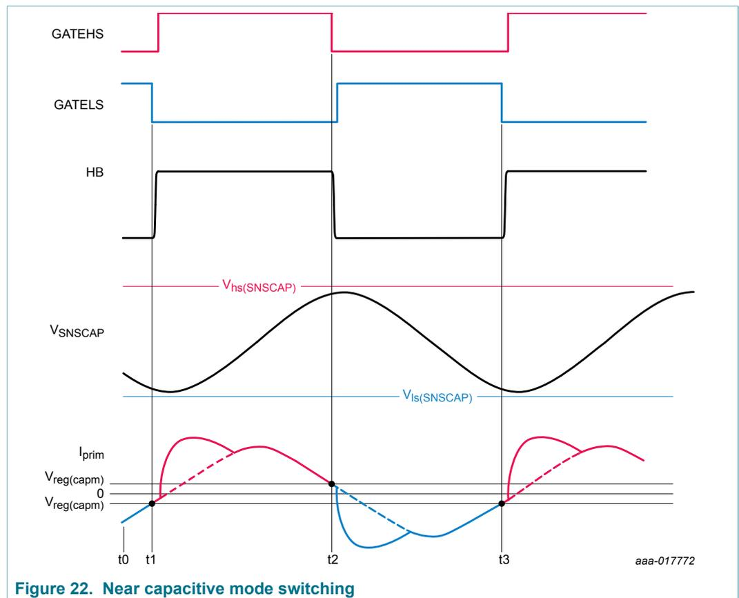
Figure 22. Near capacitive mode switching
