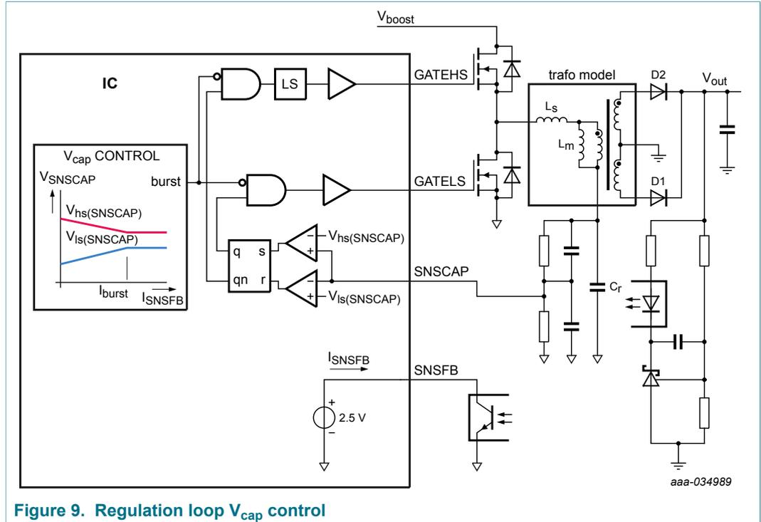
Figure 9. Regulation loop  $V_{cap}$  control
