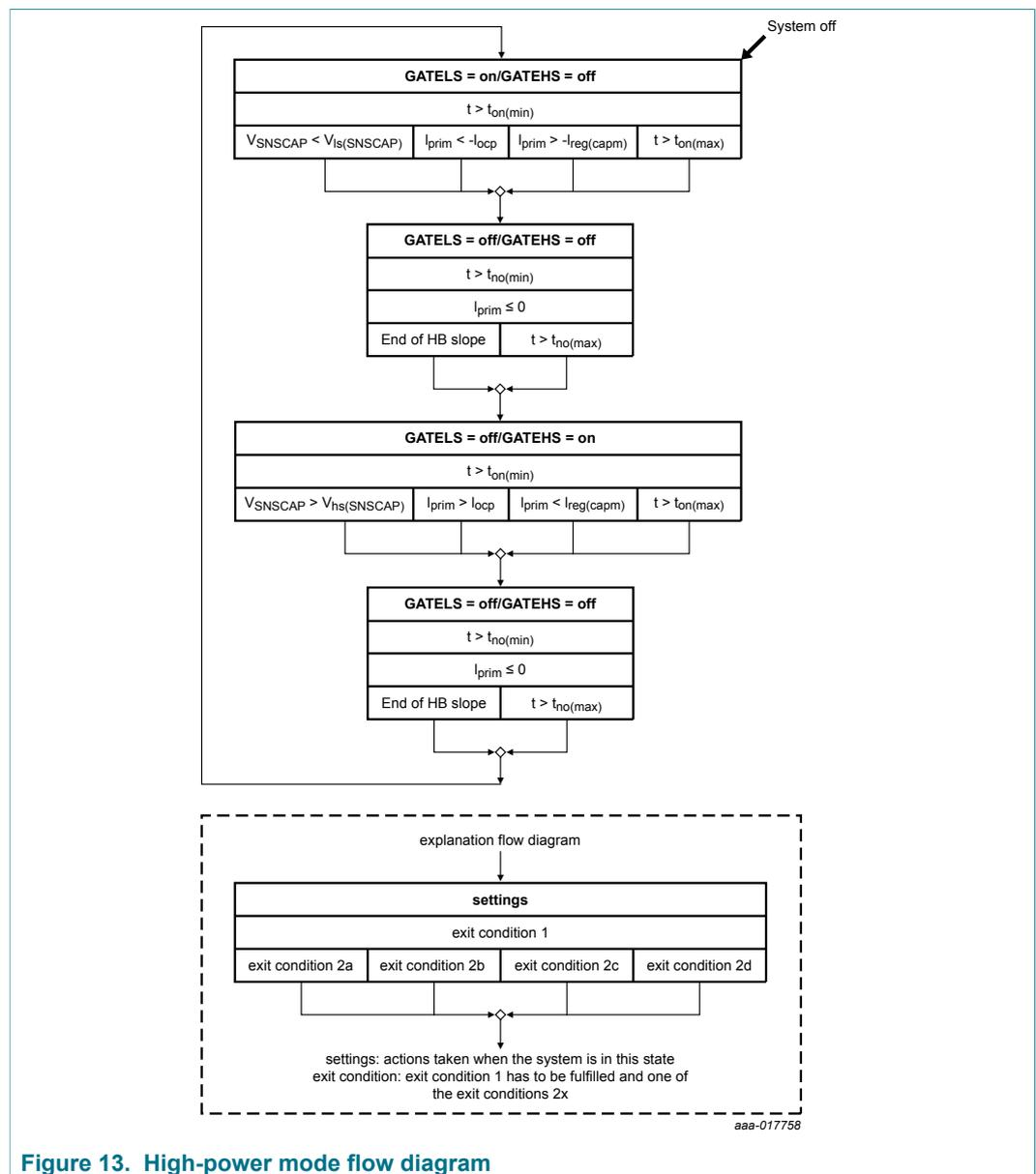
Figure 13. High-power mode flow diagram
