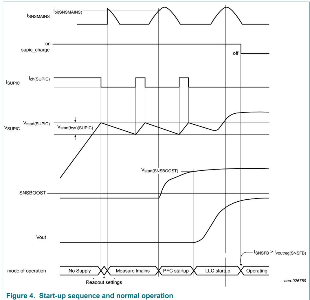
Figure 4. Start-up sequence and normal operation
