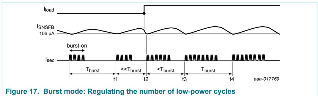
Figure 17. Burst mode: Regulating the number of low-power cycles
