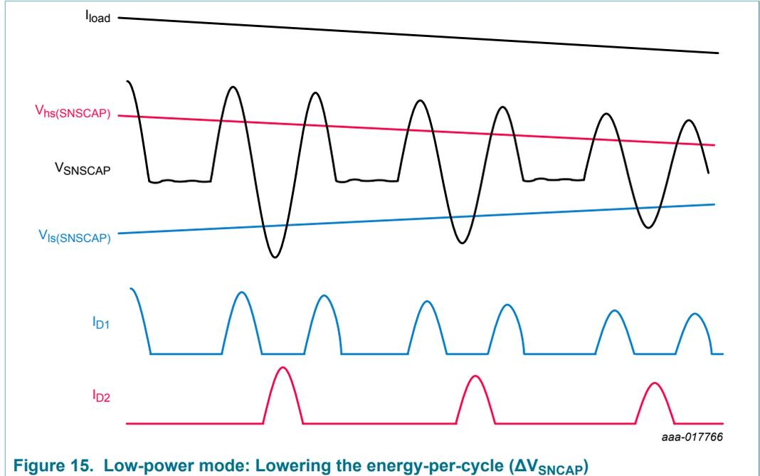
Figure 15. Low-power mode: Lowering the energy-per-cycle ( $\Delta V_{SNSCAP}$ )
