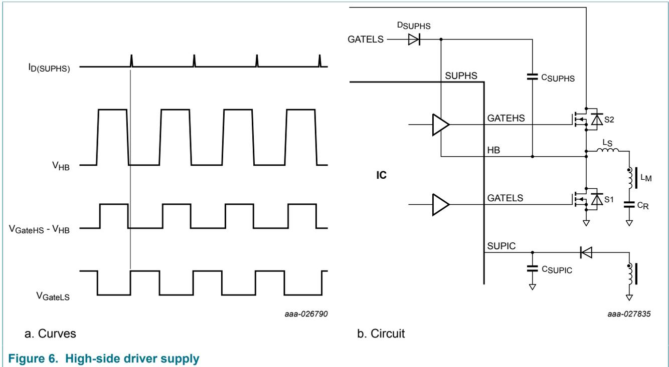
Figure 6. High-side driver supply
