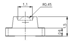
For reflow soldering (propose)
