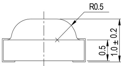
For reflow soldering (Propose)
