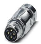
Coupler connector, straight, for standard and SPEEDCON interlock, M17, number of positions: 7+PE, type of contact: Pin, Crimp connection, shielded: yes, cable diameter range: 5 mm ... 8 mm
