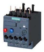
Overload relay 5.5...8.0 A Thermal For motor protection Size S00, Class 10 Contactor mounting Main circuit: Screw Auxiliary circuit: Screw Manual-Automatic-Reset
