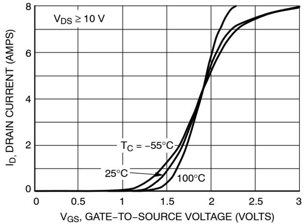
Figure 2. Transfer Characteristics
