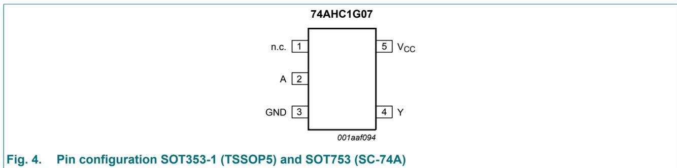
Fig. 4. Pin configuration SOT353-1 (TSSOP5) and SOT753 (SC-74A)
