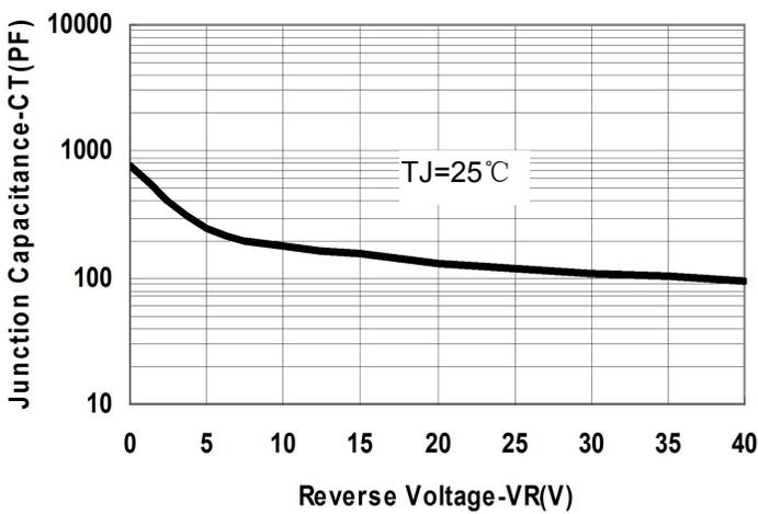
Fig.1-Typical Junction Capacitance
