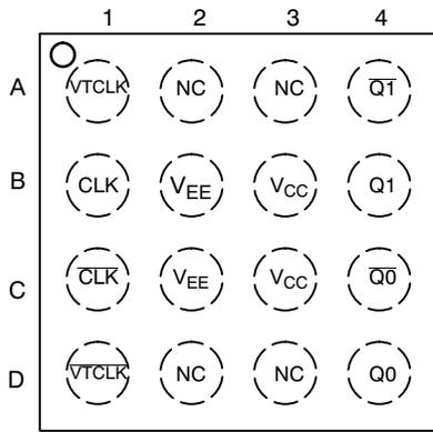
Figure 1. BGA-16 and LGA-16 Pinout (Top View)
