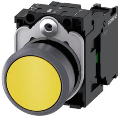
Pushbutton, 22 mm, round, plastic with metal front ring, yellow, pushbutton, flat, momentary contact type, with holder, 1 NO, screw terminal, with laser labeling, symbol number according to, ISO 7000 or IEC 60417
