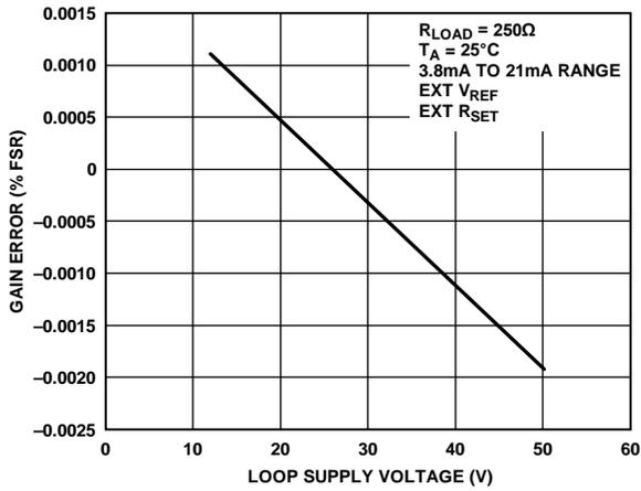
Figure 19. Gain Error vs. Loop Supply Voltage
