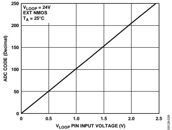
Figure 40. On-Chip ADC Code vs. V<sub>LOOP</sub> Pin Input Voltage
