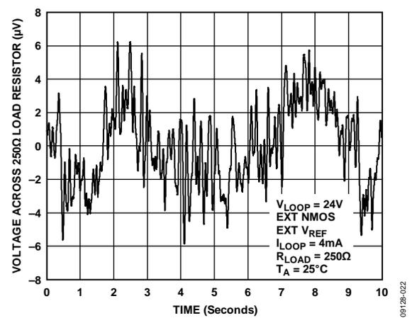
Figure 24. Loop Current Noise, 0.1 Hz to 10 Hz Bandwidth
