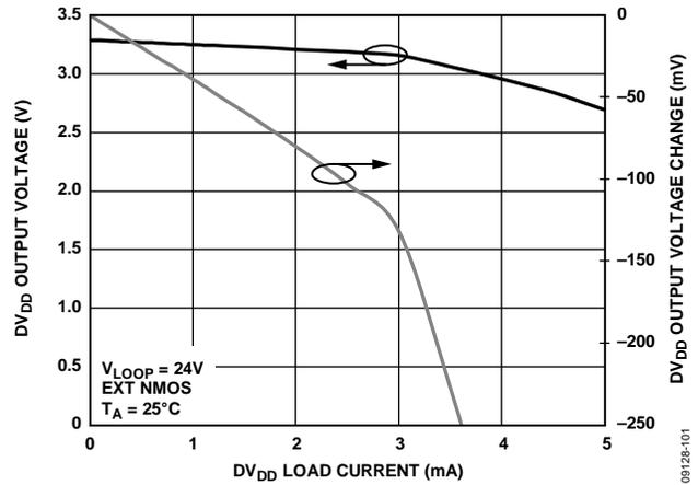
Figure 34. DV<sub>DD</sub> Output Voltage vs. Load Current
