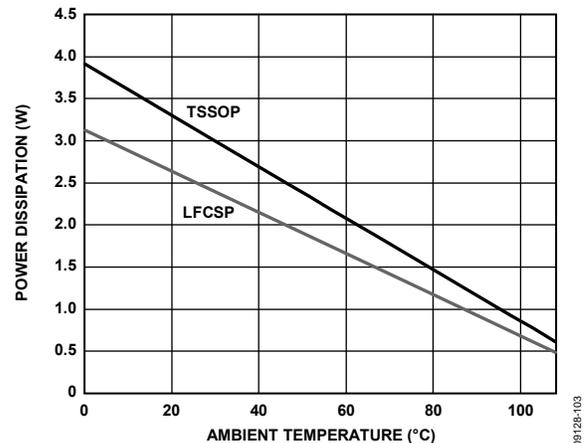
Figure 52. Maximum Power Dissipation vs. Ambient Temperature
