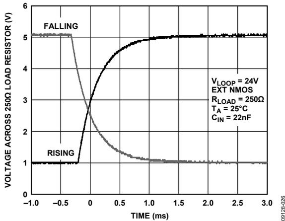
Figure 27. Full-Scale Loop Current Step,  $C_{IN} = 22nF$
