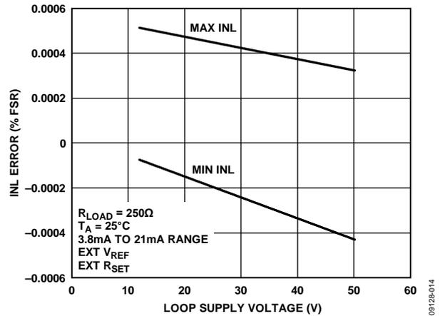
Figure 16. Integral Nonlinearity Error vs. Loop Supply Voltage
