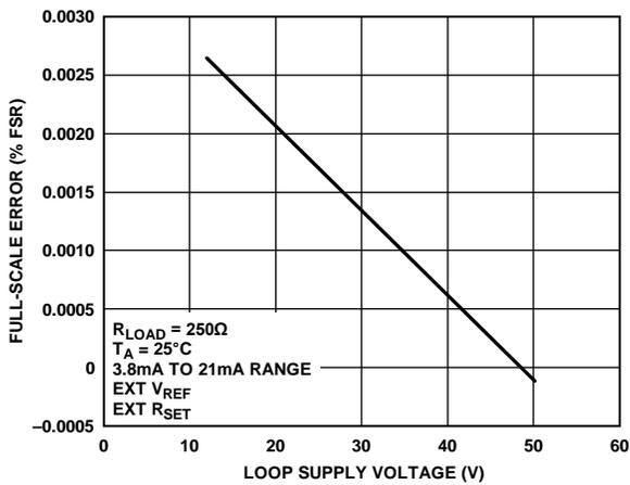
Figure 20. Full-Scale Error vs. Loop Supply Voltage
