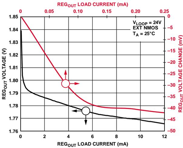
Figure 31. REG<sub>OUT</sub> Voltage vs. Load Current
