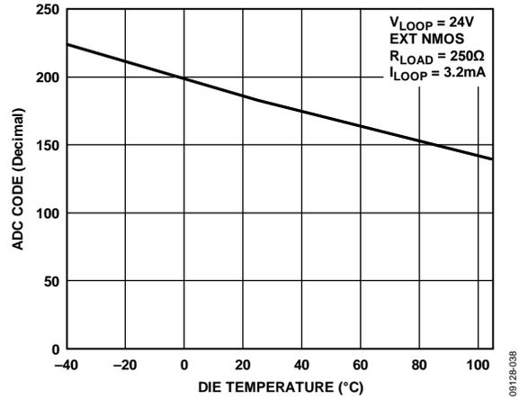
Figure 39. On-Chip ADC Code vs. Die Temperature
