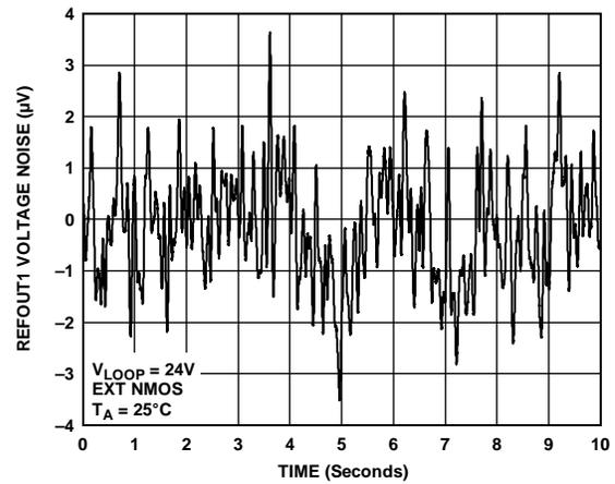
Figure 35. REFOUT1 Voltage Noise, 0.1 Hz to 10 Hz Bandwidth
