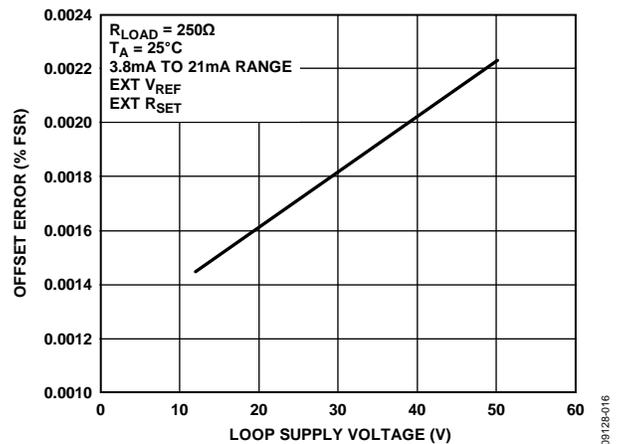
Figure 18. Offset Error vs. Loop Supply Voltage
