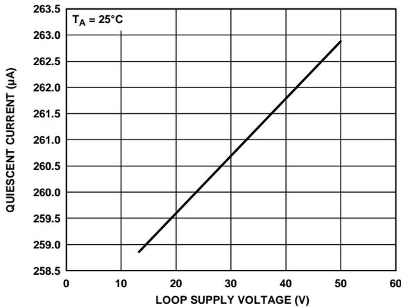
Figure 32. Quiescent Current vs. Loop Supply Voltage
