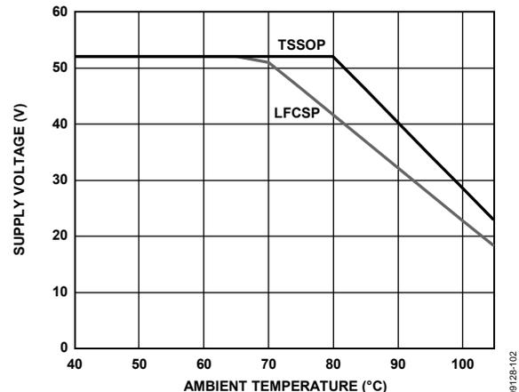
Figure 53. Maximum Supply Voltage vs. Ambient Temperature
