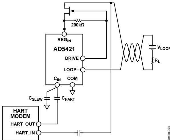
Figure 47. Connecting a HART Modem to the AD5421
