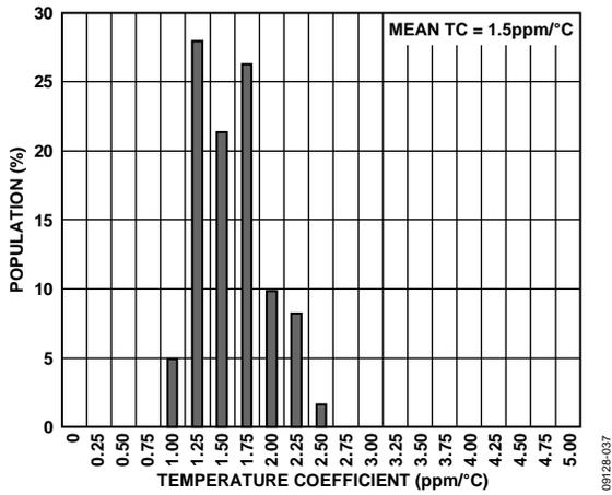
Figure 38. REFOUT1 Temperature Coefficient Histogram (C Grade Device)
