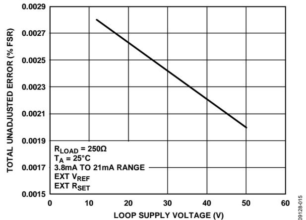
Figure 17. Total Unadjusted Error vs. Loop Supply Voltage
