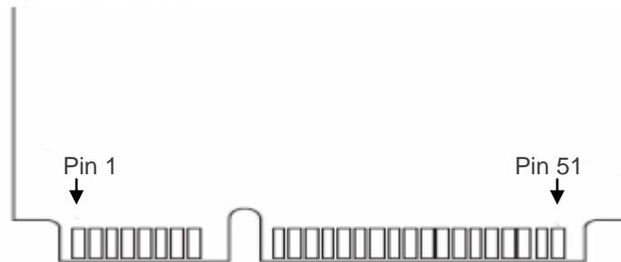
Figure 1-1 Pin Assignment
