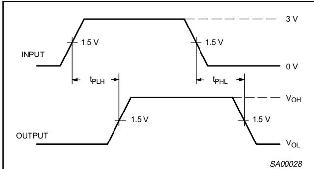
$t_{PLH}$  and  $t_{PHL}$  are the same as  $t_{pd}$ .
