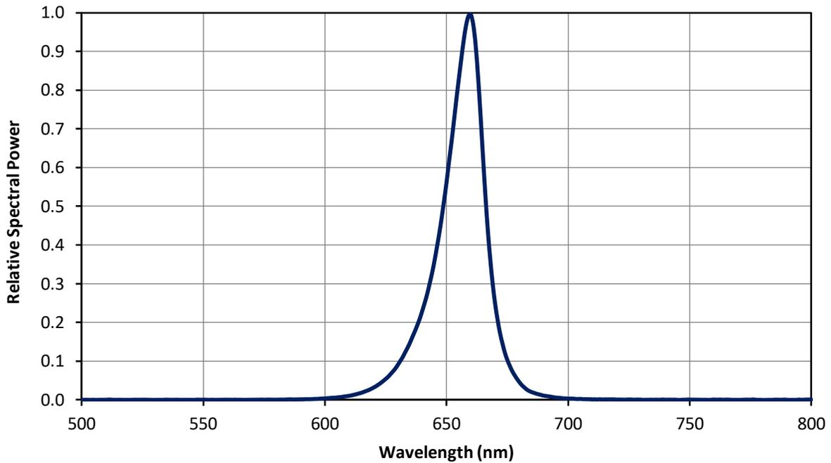
Figure 5: Relative spectral power vs. wavelength @  $T_c = 25^\circ\text{C}$ .
