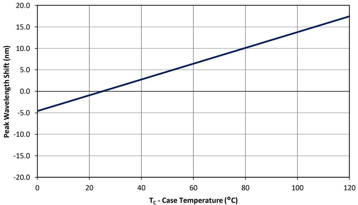
Figure 10: Typical peak wavelength shift vs. case temperature.
