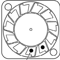
Note: The glue on the impeller is for impeller balance. Please don't remove it.
