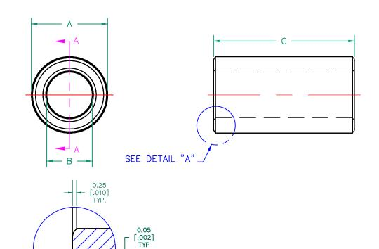
DETAIL "A" CHAMFER SCALE=6:1
